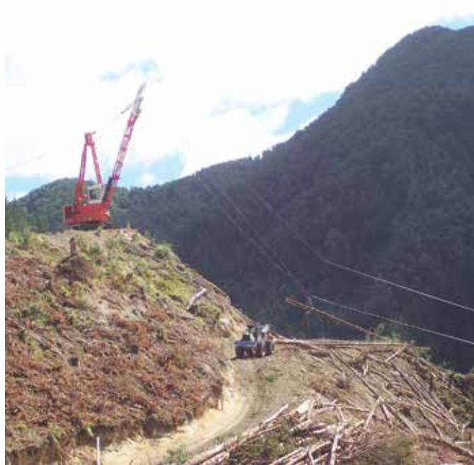
Split-level landing with stems two-staged back to a processing site
