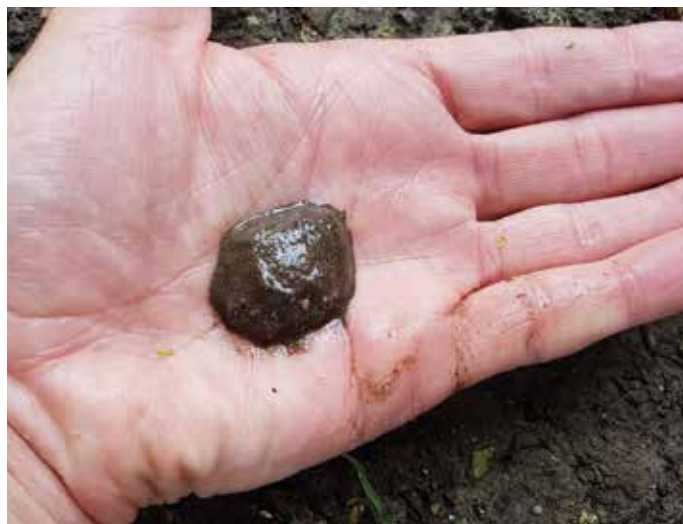
Left: The process of rolling a worm is a simple test for clay content. Right: The pat and tap test for silt
