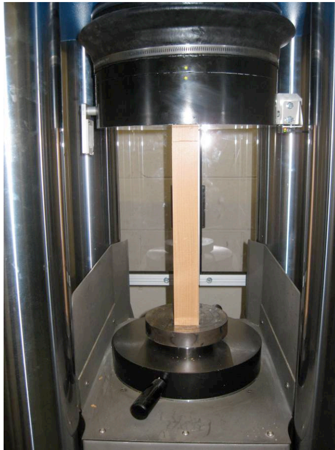
Figure 4. Typical Testing Configuration for Compression Parallel-to-Grain Specimens
