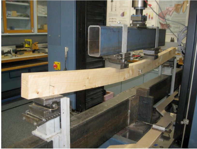
Figure 1. Typical Testing Configuration for Flexure Specimens (Note: Deflection Yoke Shown in Lower Right Removed as Specimens Nearing Failure)
