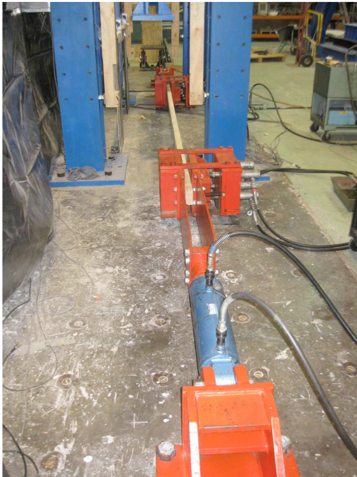
Figure 3. Typical Testing Configuration for Tension Parallel-to-Grain Specimens
