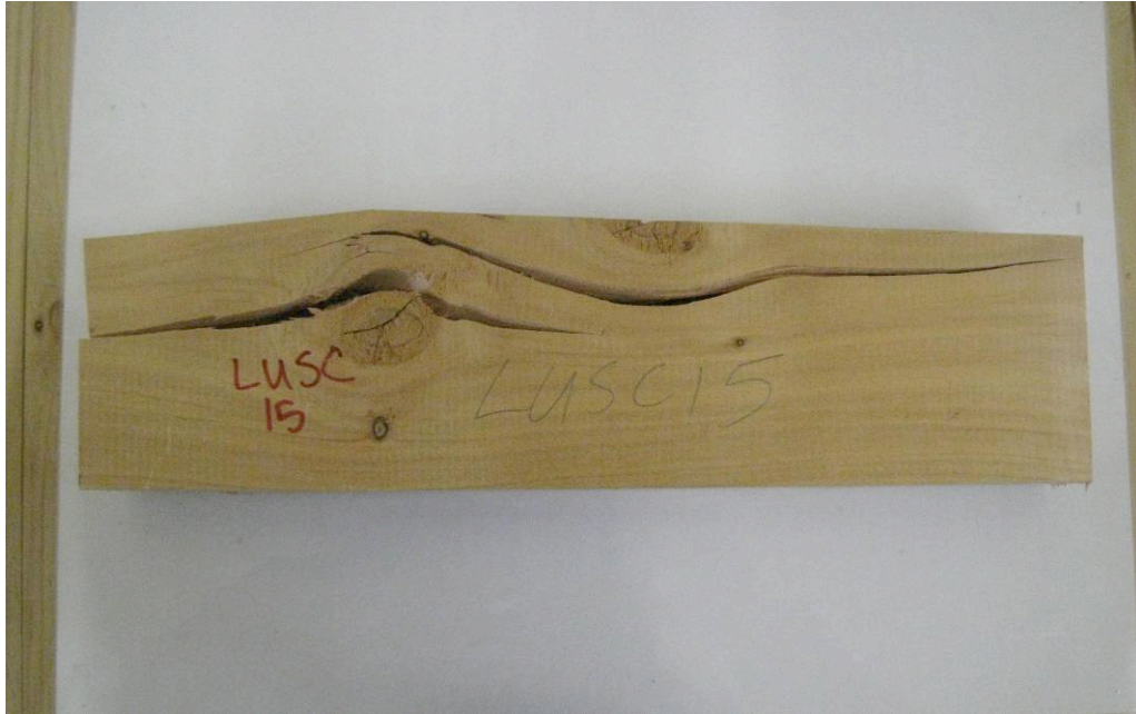
Figure 5. Example of Crushing and Splitting Failure Observed in Some Compression Parallel-to-Grain Specimens
