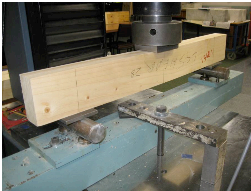
Figure 2. Typical Testing Configuration for Beam Shear Specimens
