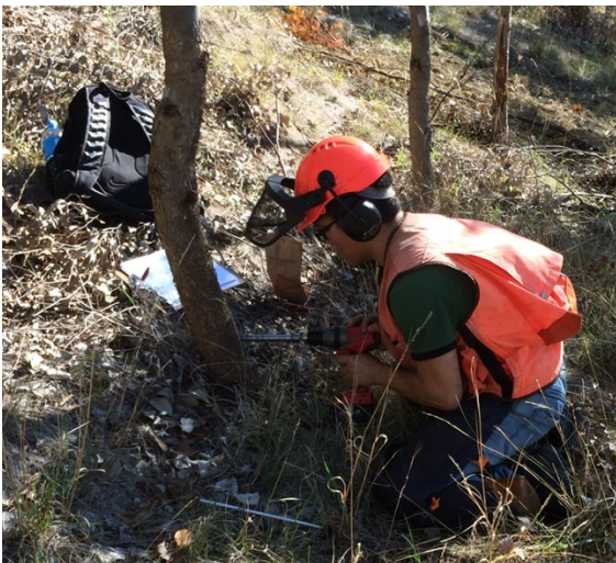
Figure 1: Top: Probing of an E. bosistoana tree with the battery powered corer developed for this project. Bottom: Corer and core.
