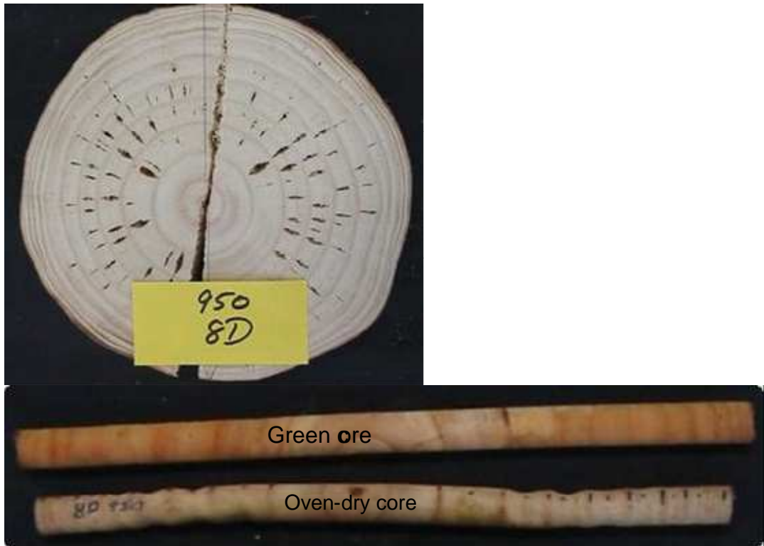
Example of severely checked disc compared with a green and oven-dry core from the same tree
