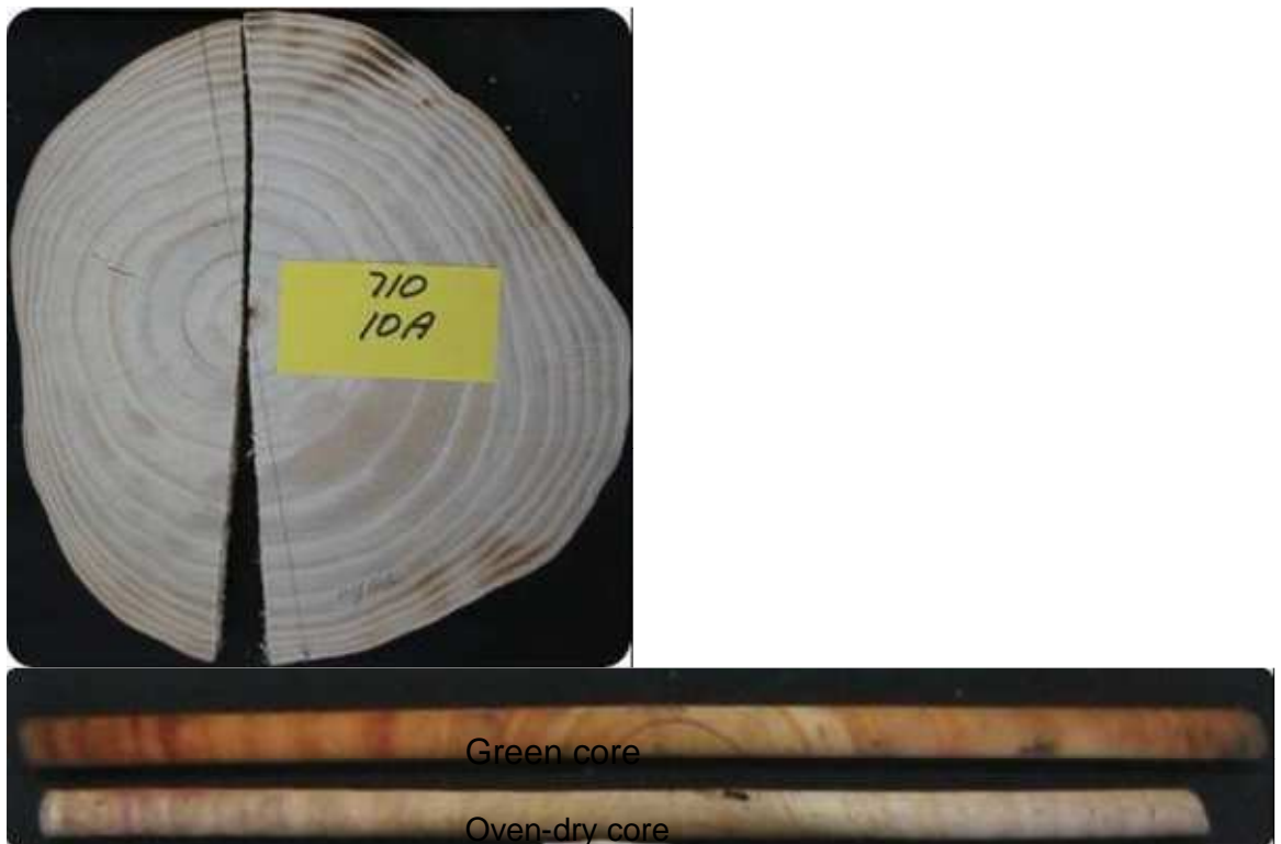
Example of a non-checked disc compared with a green and oven-dry core from the same tree
