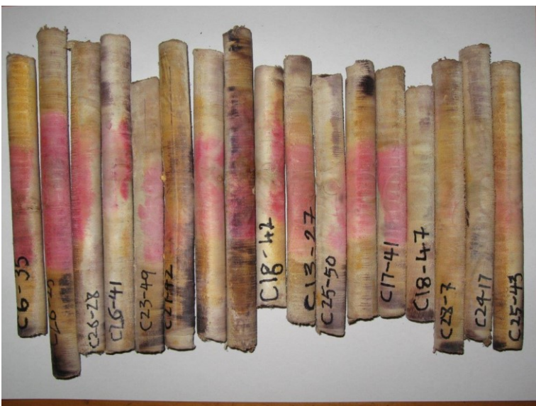
Figure 1: E. bosistoana cores stained with methyl orange. Heartwood is highlighted pink.
