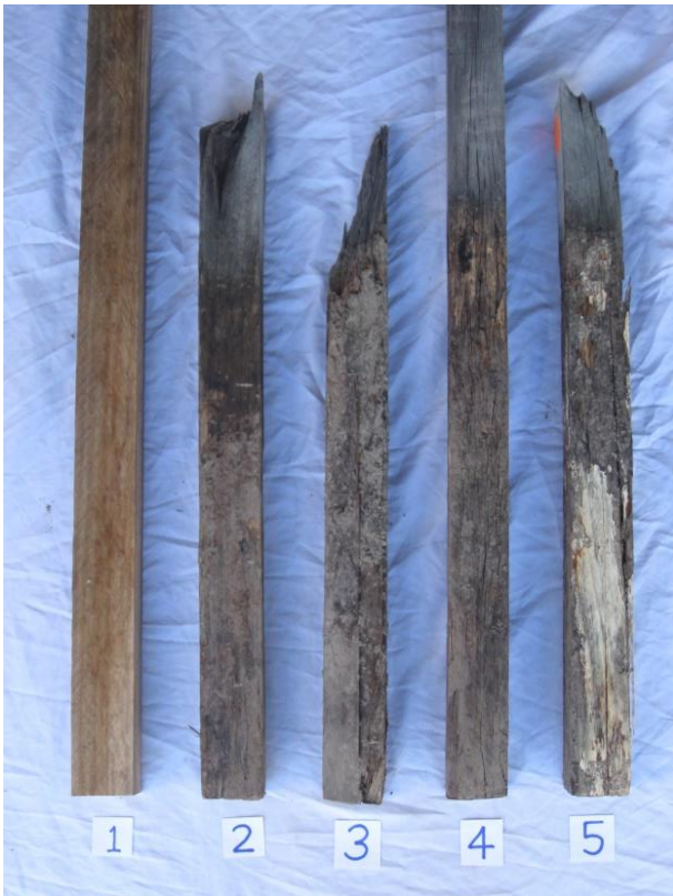
Figure 19: Sections of E. bosistoana posts with no. 1 unused timber and no's 2,3,4 & 5 all sections of broken posts dug out of vineyard 1 after 10 years in ground. Note no. 5 is pith wood.
