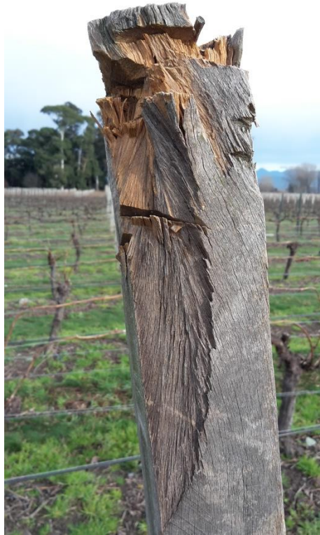
Figure 18: E. bosistoana showing repeated damage by machine harvester in vineyard 1.
