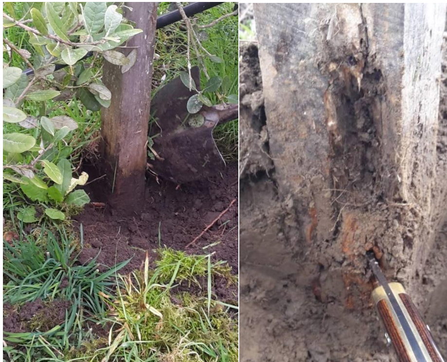
Figure 9: E. globoidea posts after 10 years in service. Post 116 in feijoa orchard at vineyard 3 showing no sign of decay and failed post 62 at vineyard 2. Note: Post 62 showed the severest decay of all assessed E. globoidea posts.
