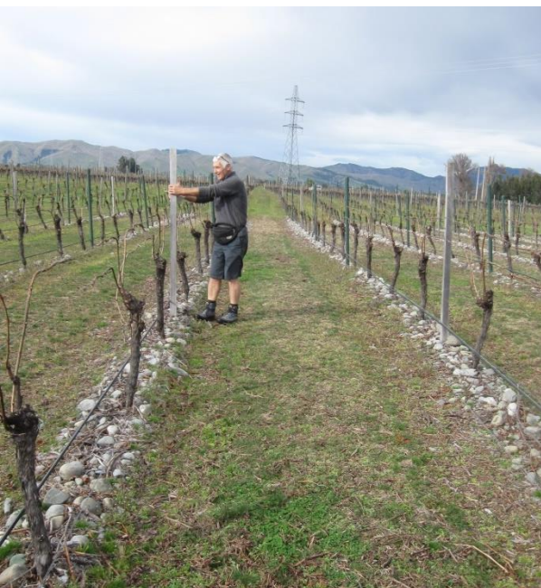
Figure 15: In service assessment using the 'pull' test at vineyard 1.
