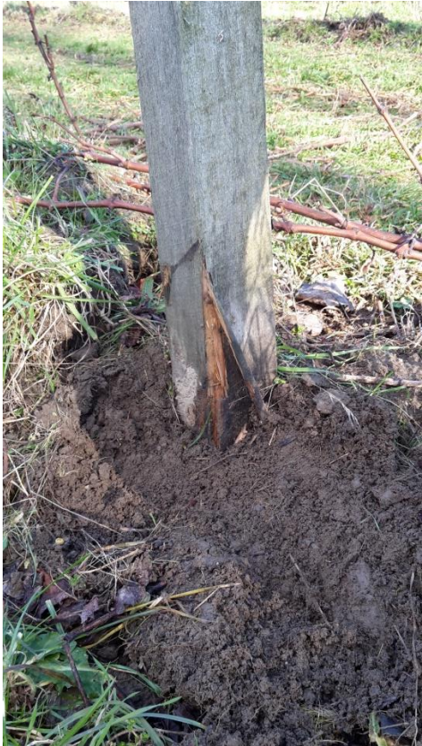
Figure 21: E. globoidea post with recent damage by mechanical undervine cultivation in vineyard 2.
