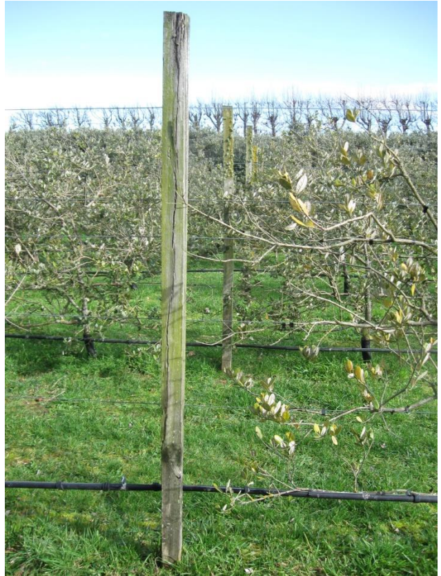
Figure 22: E. globoidea post in feijoa orchard. This one is sawn through the centre of the stem as the line of the pith is evident.
