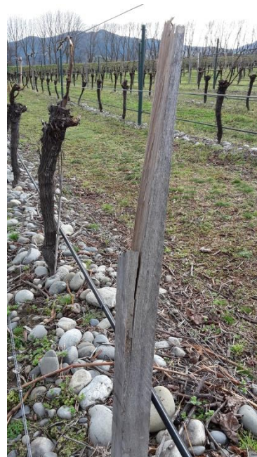
Figure 16: E. bosistoana post broken by machine harvester in vineyard 1.
