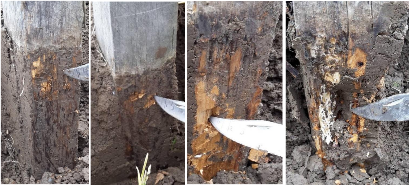
Figure 6: Range of decay in E. bosistoana posts after 10-11 years in service. From left to right: < 2mm; 2-5 mm; 10-20 mm; > 30mm (post 10, 21, 40 and 41). Note: post 41 showed the severest decay of all assessed E. bosistoana posts.
