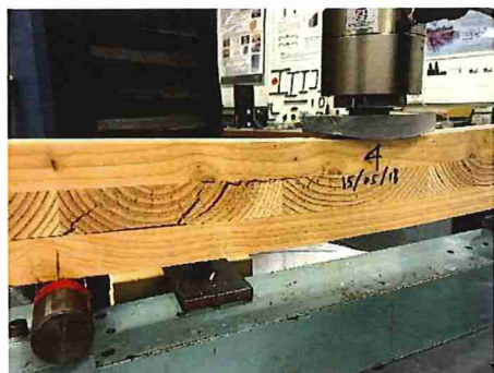
Figure 9: Specimen failed in rolling shear (left)
