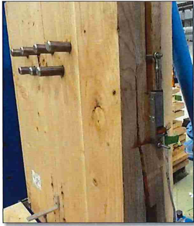
Figure 20: CLT5 - Tensile Splitting
