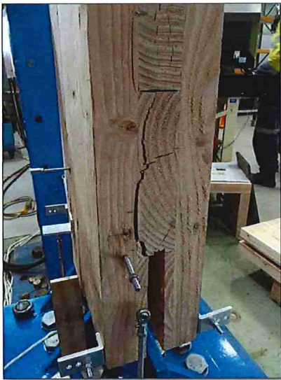
Figure 14: CLT45 Tensile Splitting
