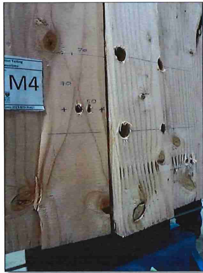
Figure 22: Dowelled CLT5 connections with screws
