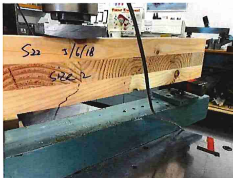
Figure 10: Specimen failed in tension of bottom edge
