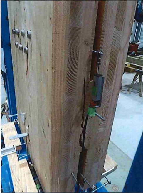
Figure 25: CLT7 Tensile Splitting
