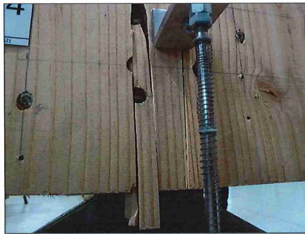
Figure 18: CLT45 Row Shear Failure
