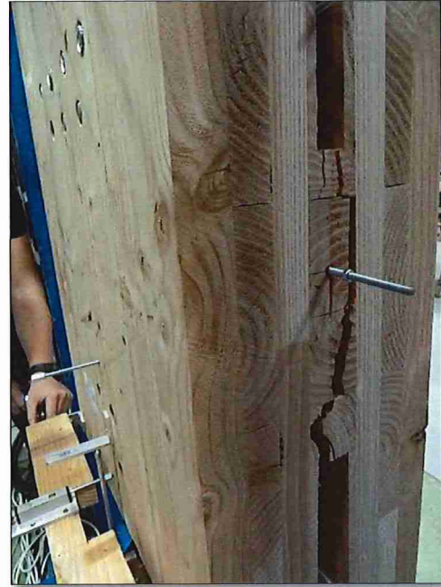
Figure 26: CLT7 Tensile Splitting
