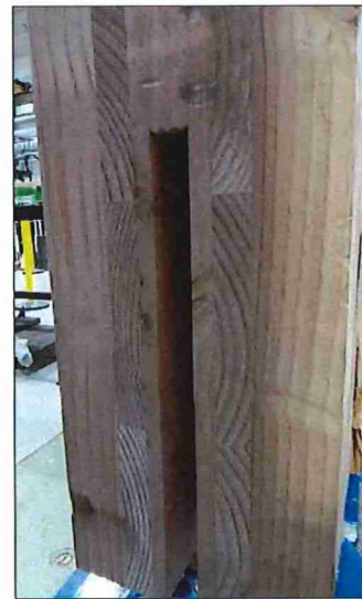
Figure 23: Ultimate failure without tensile splitting
