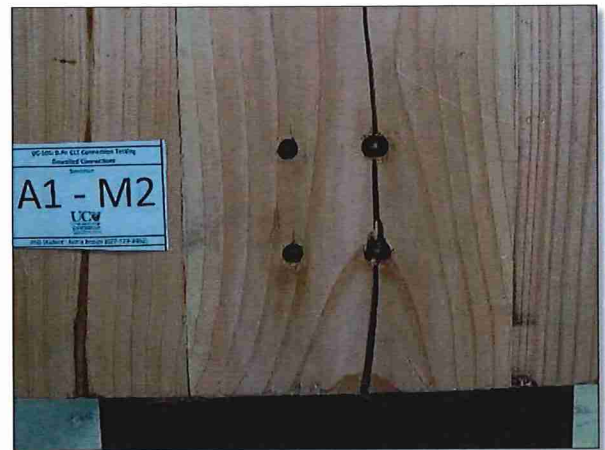
Figure 15: CLT45 Row Shear
