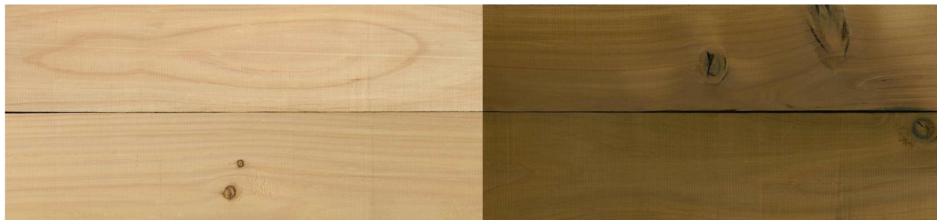
Figure 11. Photographs of board surfaces before (left) and after (right) modification. For each image, the top board is predominantly heartwood and the bottom board predominantly sapwood.
