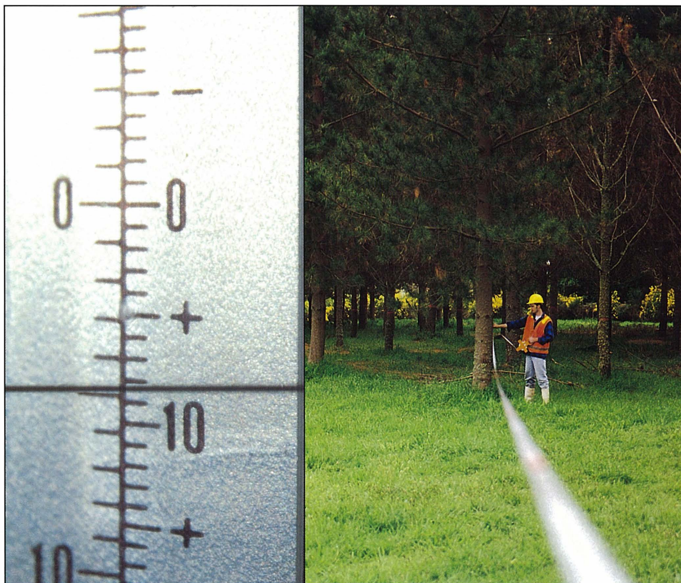
Figure 8. Percentage scale and length tape method. Percentage scale on right is 8% ( 5^\circ on left scale).
