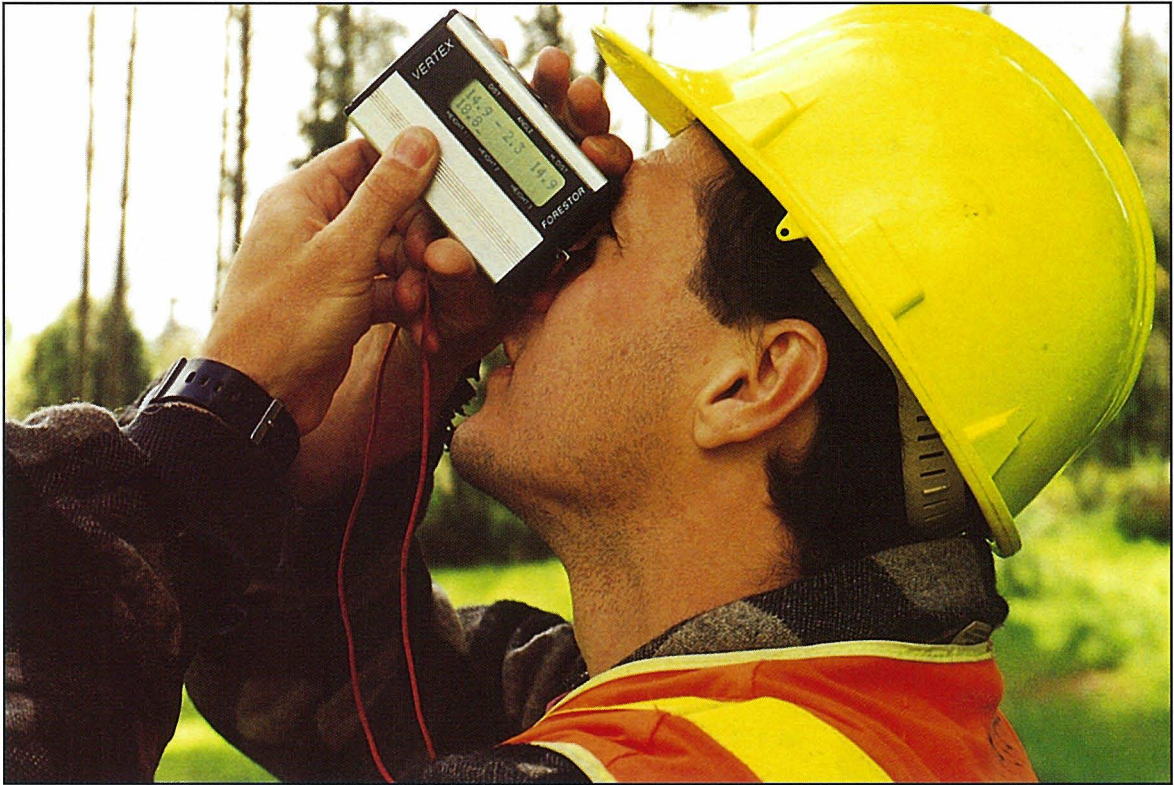
Figure 14. The Forestor VERTEX electronic hypsometer. This uses ultrasonic technique for measuring distance.
