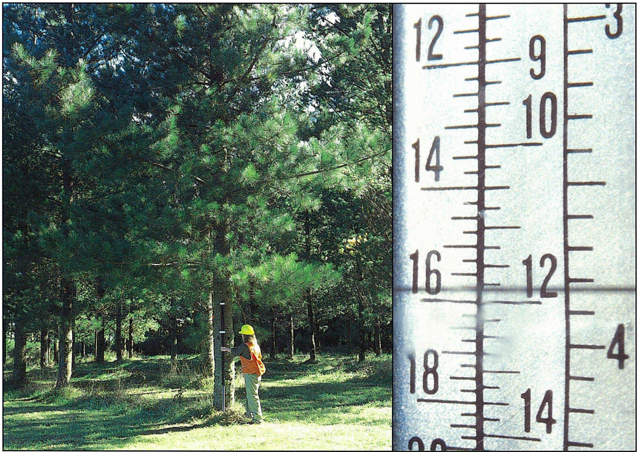
Figure 12. Degrees scale and adjustable target staff method. Degrees scale on right reads 38^\circ . Scales on left are for fixed distances of 15 m and 20 m, right to left.
