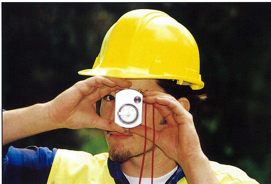
Figure 10. Observer looks through prism at target staff
