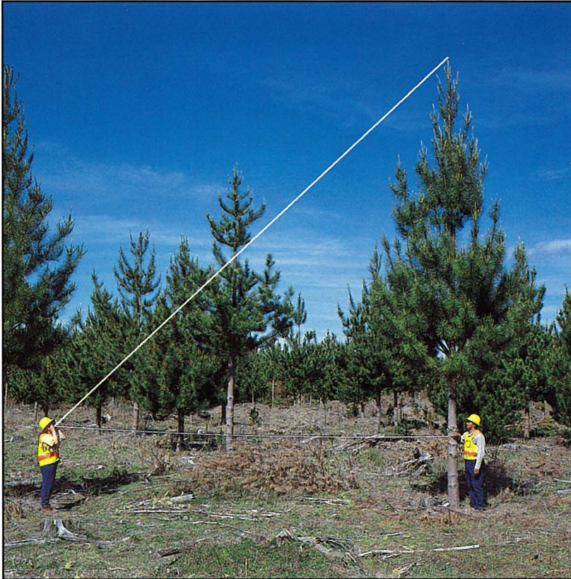
Figure 7. Degrees scale and length tape method.
