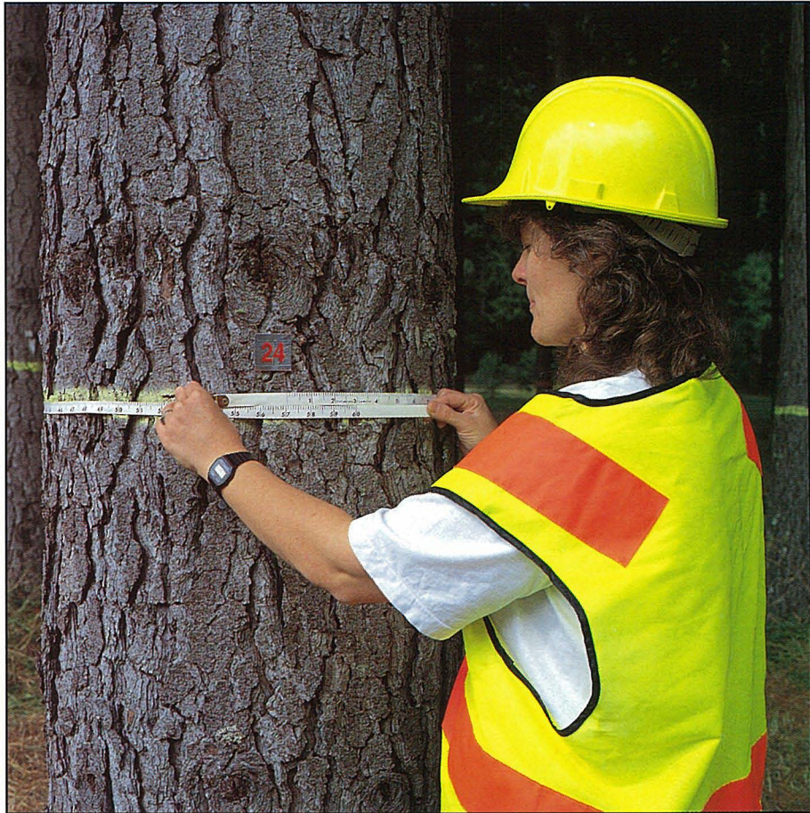
Figure 1. dbh is measured over the breast height band of the tree or at 1.4 m above ground level . This dbh is 57.1 cm.
