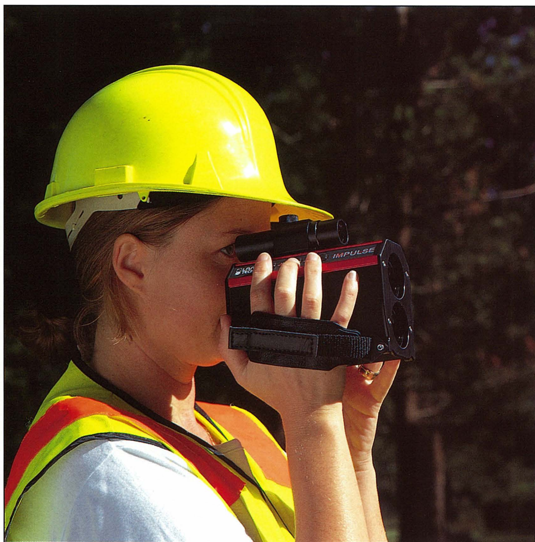
Figure 15. The Laser Technology IMPULSE electronic hypsometer. This uses a laser technique to measure distance.
