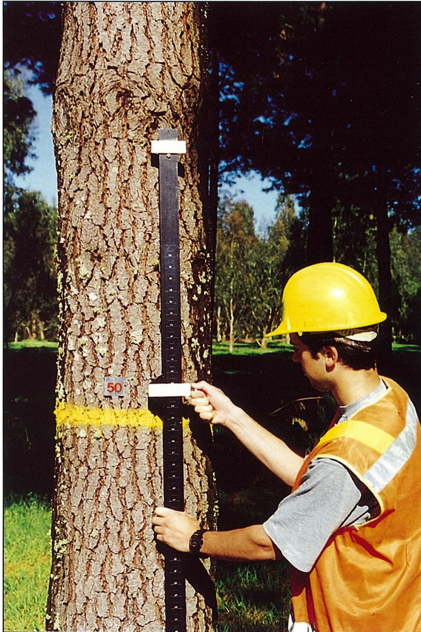
Figure 13. Percentage scale and adjustable target staff method.
