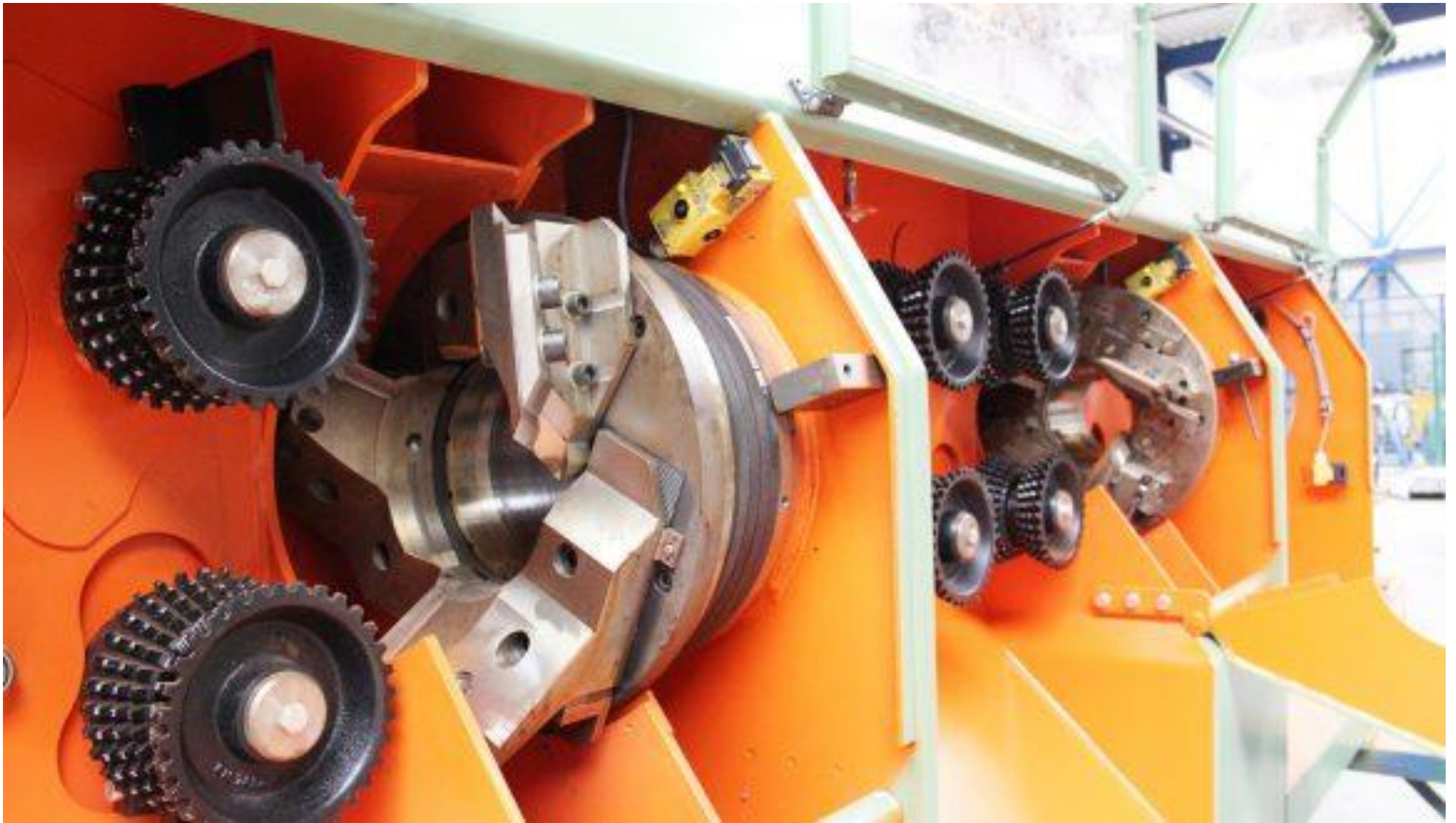
Figure 14: Rounding / dowel machines www.bezner-oswald.com . A video of the machine in operation can be seen at https://youtu.be/KJVEsVWf4LY .
