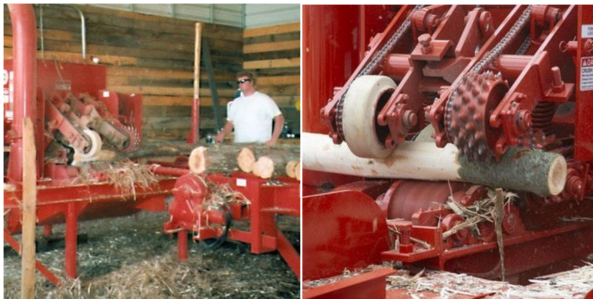
Figure 10: Higher capacity automated stationary 'rosser head type' pole peeler from www.morbark.com . A video of the machine in operation can be seen at https://www.youtube.com/watch?v=t5mVVhd8Vfw .
