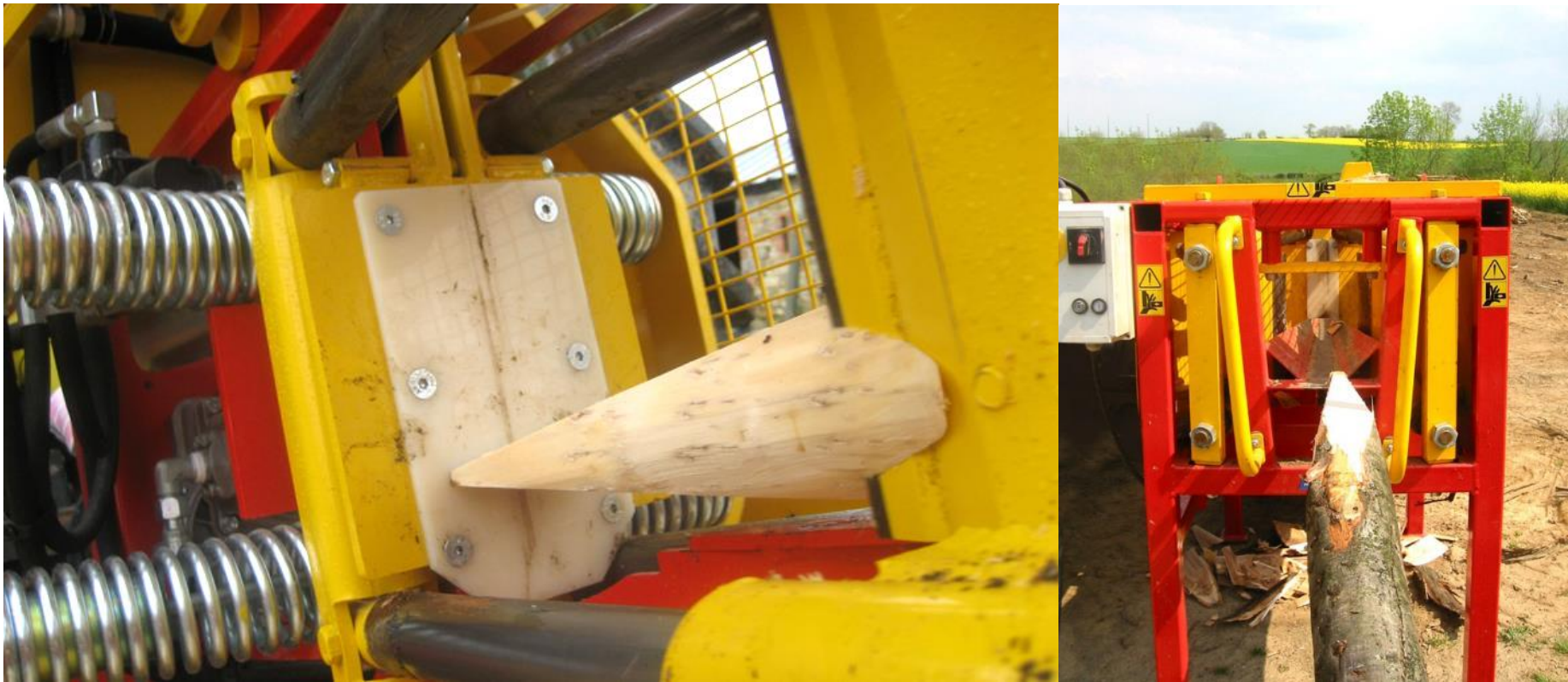
Figure 19: Pointing machine using hydraulic driven blades from www.rabaud.com/en/products/forestry-machines . A video of the machine in operation can be seen at https://youtu.be/oqanPty8Ems .
