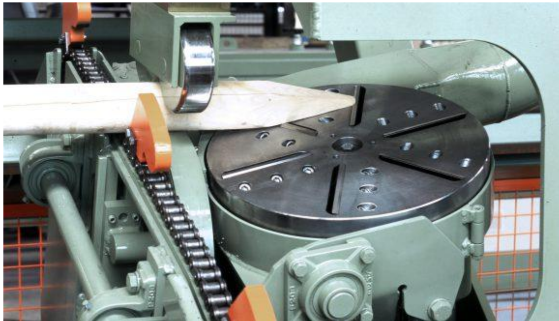
Figure 20: Pointing and chamfering machine from https://www.bezner-oswald.com/products/chamfering-pointing-machine/ (left) and http://www.brodbaek.dk/Files//Billeder/Brodbaek/Datablade_PDF/Engelsk/64.002%20Post%20Pointing%20160215.pdf .
