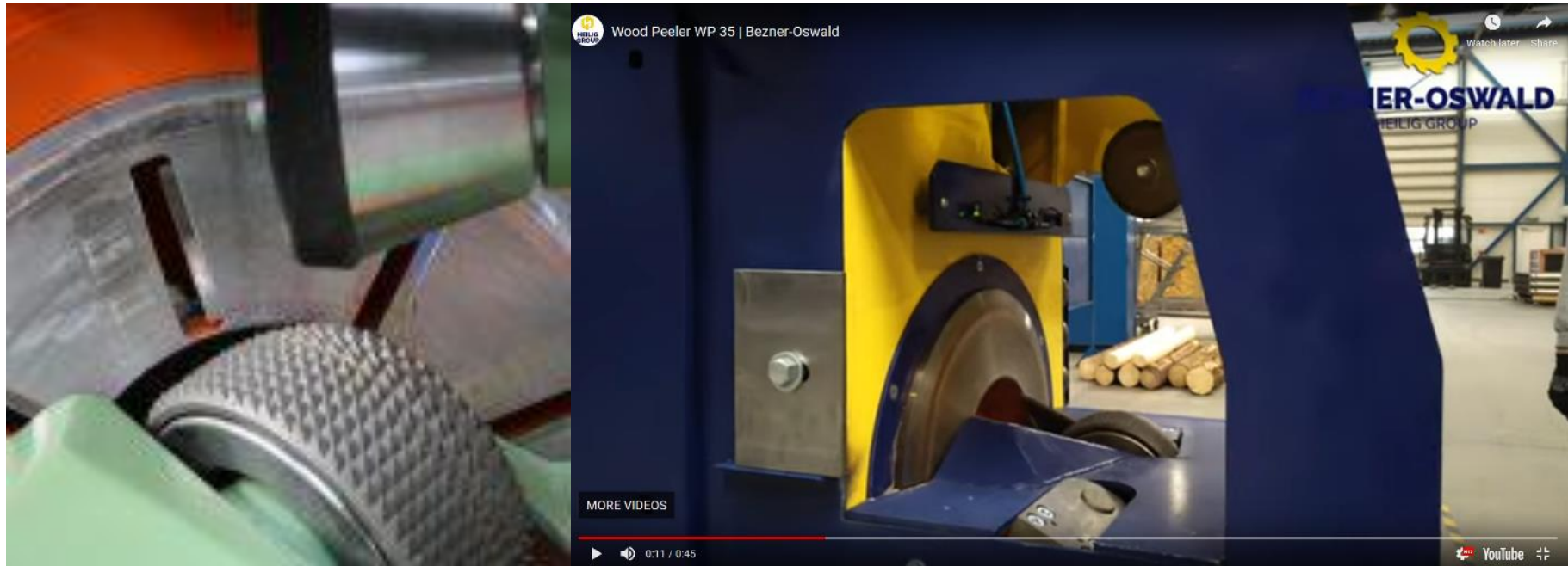
Figure 9: Higher capacity automated stationary 'disc type' post peeler from www.bezner-oswald.com/ . A video of the machine in operation can be seen at https://youtu.be/NVIWaf1ayI .
