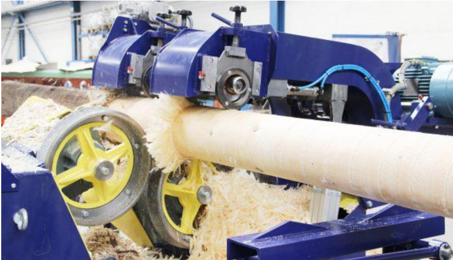
Figure 11: Higher capacity automated stationary 'rosser head type' pole peeler from www.bezner-oswald.com . A video of the machine in operation can be seen at https://youtu.be/HX_5qIZUtLM?t=37 .
