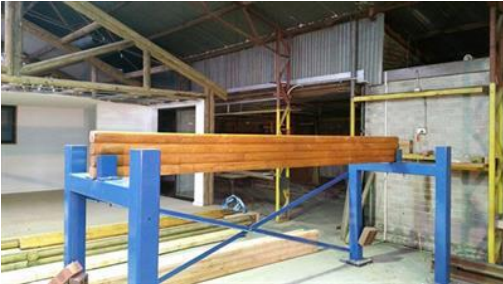
Figure 26: Patented composite beam made from peeler cores by www.loggo.com.au . A video of the LOGGO system can be found at https://vimeo.com/54001004 .
