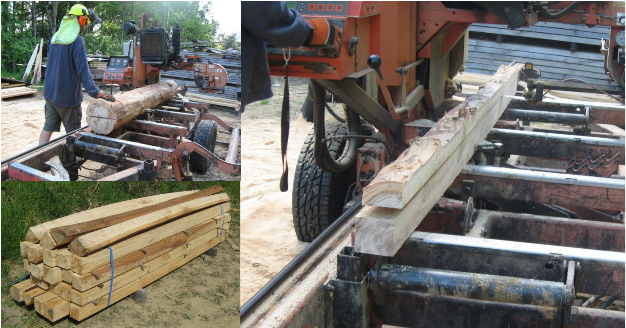
Figure 18: Sawing 4 square heartwood posts from larger diameter durable eucalypt logs with a mobile horizontal bandaw. Note the distortion during sawing due to growth stresses.
