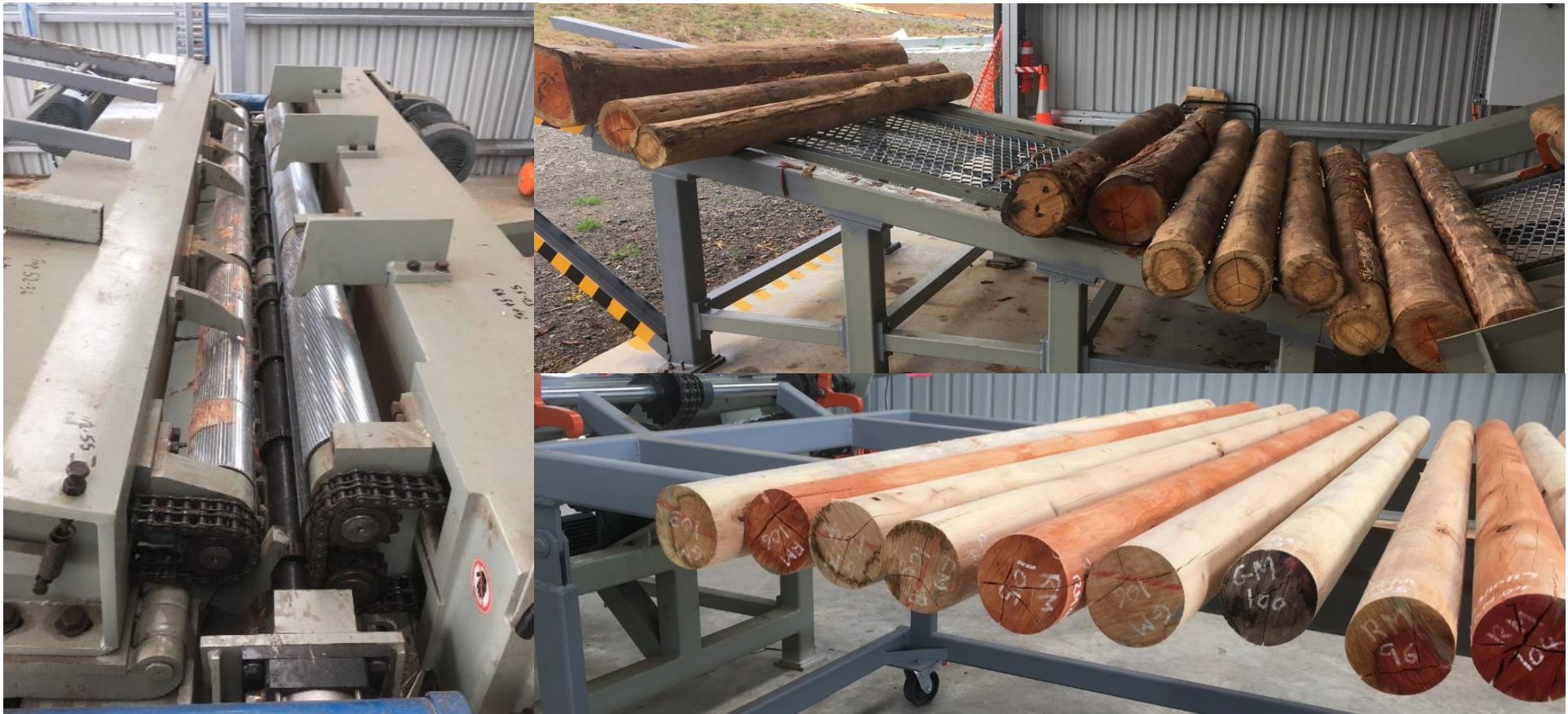
Figure 15: Spindle less lathe used for eucalypt post manufacturing by www.superforestplantations.com.au/ . Log length up to 2.5m; diameter range 80 – 400 mm. Lathe requires debarked logs (220 mm above bark for 100 mm heartwood post from commercial thinning. 250 posts / day. Now tested for durability and strength. $40/post ($14/m for 2.6m posts) (Lausberg, 2019).
