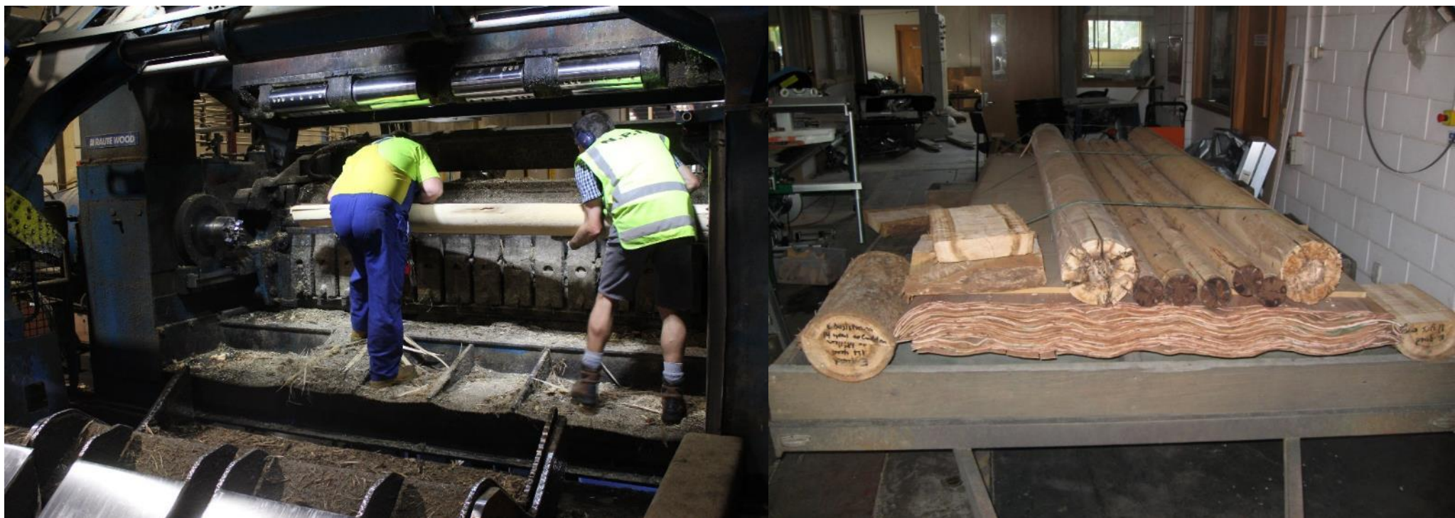
Figure 16: Peeling of durable NZDFI eucalypt for veneer 2019 at NPI Ltd for a SWP project (left). Dry veneers and peeler cores (right).
