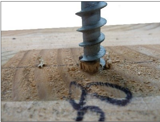
Figure 8: Shear cylinder failure in CLT narrow face 0° screw withdrawal test
