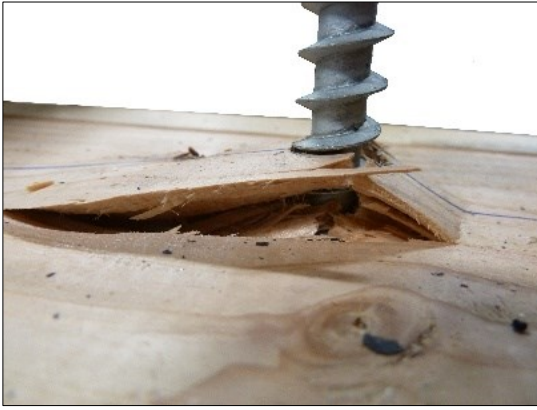
Figure 7: Timber splitting in CLT wide face 90° screw withdrawal test
