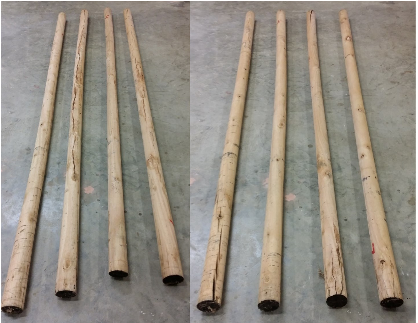
Figure 11: Dried peeler cores from an E. bosistoana and E. quadrangulata peeling trial (Altaner et al., 2019). While there was some splitting (the cores have been rotated by 180° around their axis between the left and right picture), the cores were straight and appear usable as agricultural post.
