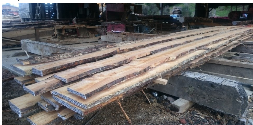
Fig 14: Boards sawn from young unpruned cypress, ready to be re-sawn, air-dried and then graded.
