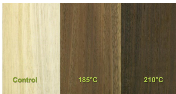
Fig 5: Thermally modified E. nitens , showing different outcomes from treatment at different temperatures.
