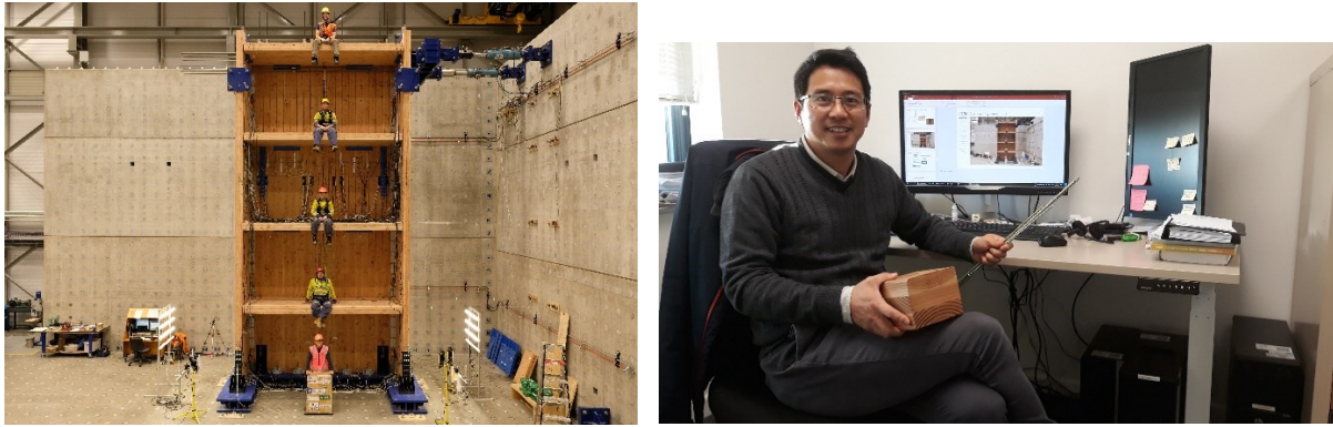
Fig 3:(left) The Douglas-fir CLT structure being tested in the University of Canterbury engineering lab (right) Dr Minghao Li with a sample of screws used to connect the CLT panels.
