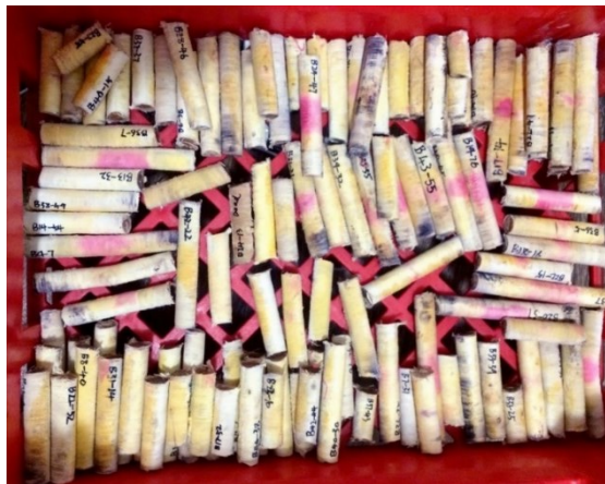
Fig 7: Stem cores showing heartwood stained pin).
