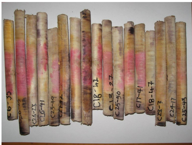
Figure 1 Staining E. bosistoana cores with methyl orange highlighted heartwood pink. (Note these cores are from a previous trial)
