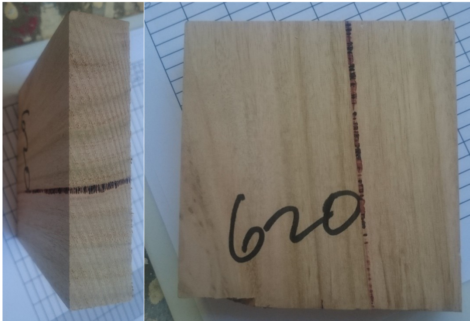
Figure 3. End grain and one face of a board with a typical kino vein.
