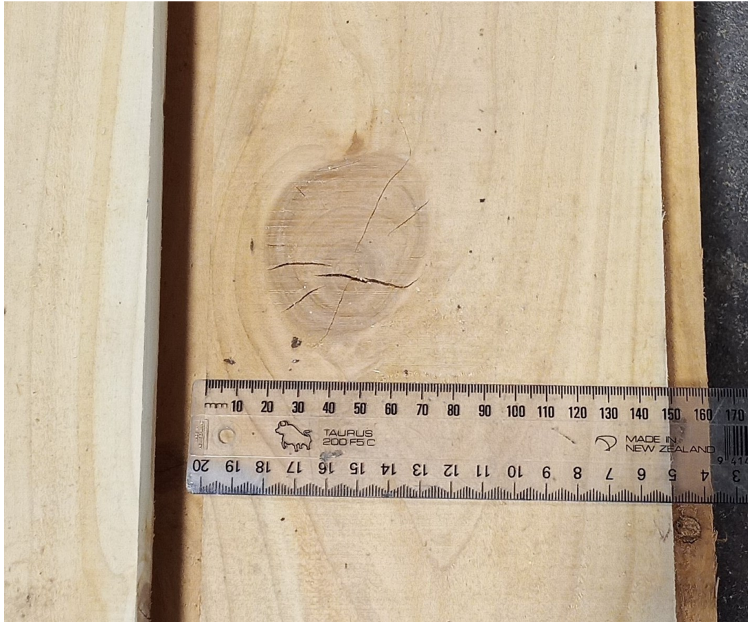
Figure 1: Large knot that is permissible for No. 1. Framing grade in a 150mm wide board but would no longer be permissible if the board was re-sawn to 100mm wide.
