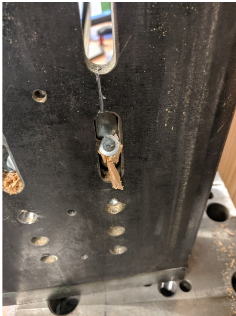
Figure 5 – Example of fully threaded screw tensile failure at the timber to steel interface.
