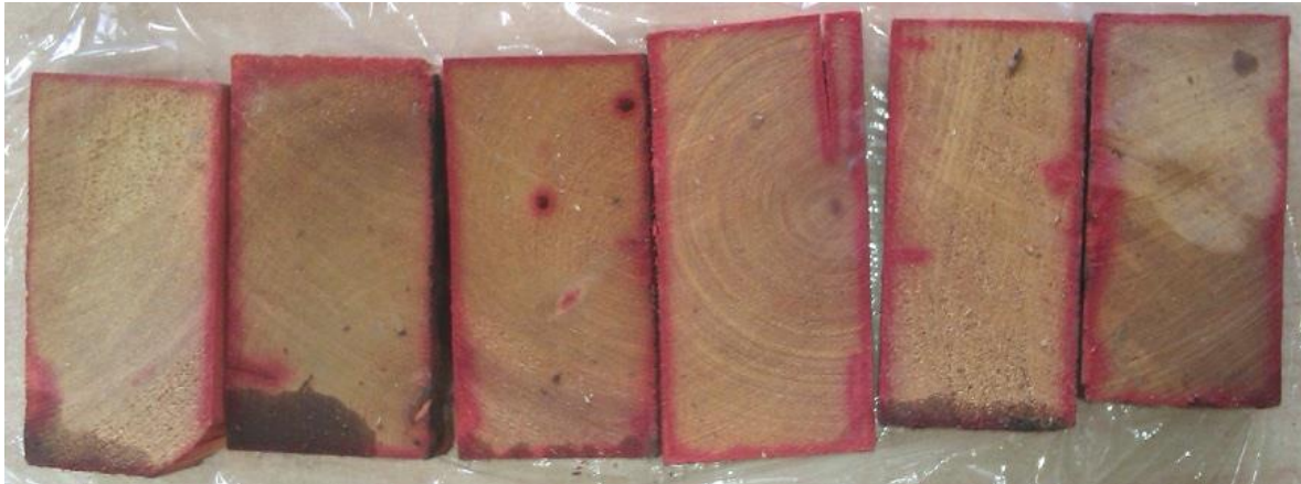
Farm-totara treatment 1: 1st set point 18kPa (20 secs), 2nd set point 65 kPa (70 secs), final vacuum -85 kPa (6 mins)
