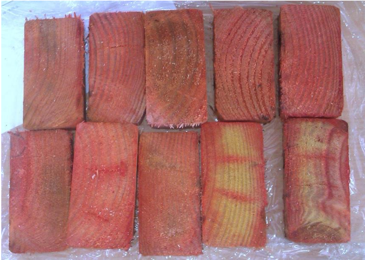
Example of Radiata pine 90x45 framing: 1st set point 18kPa (20 secs), 2nd set point 55 kPa (65 secs), final vacuum -85 kPa (6 mins)
