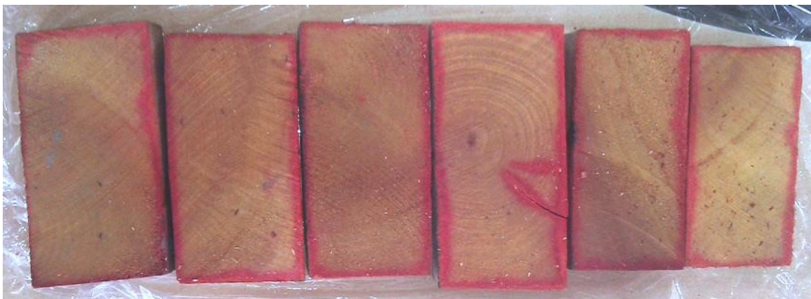
Farm-totara treatment 2: 1st set point 18 kPa (20 sec), 2nd set point 55 kPa (65 secs), final vacuum -85kPa (6 mins)
