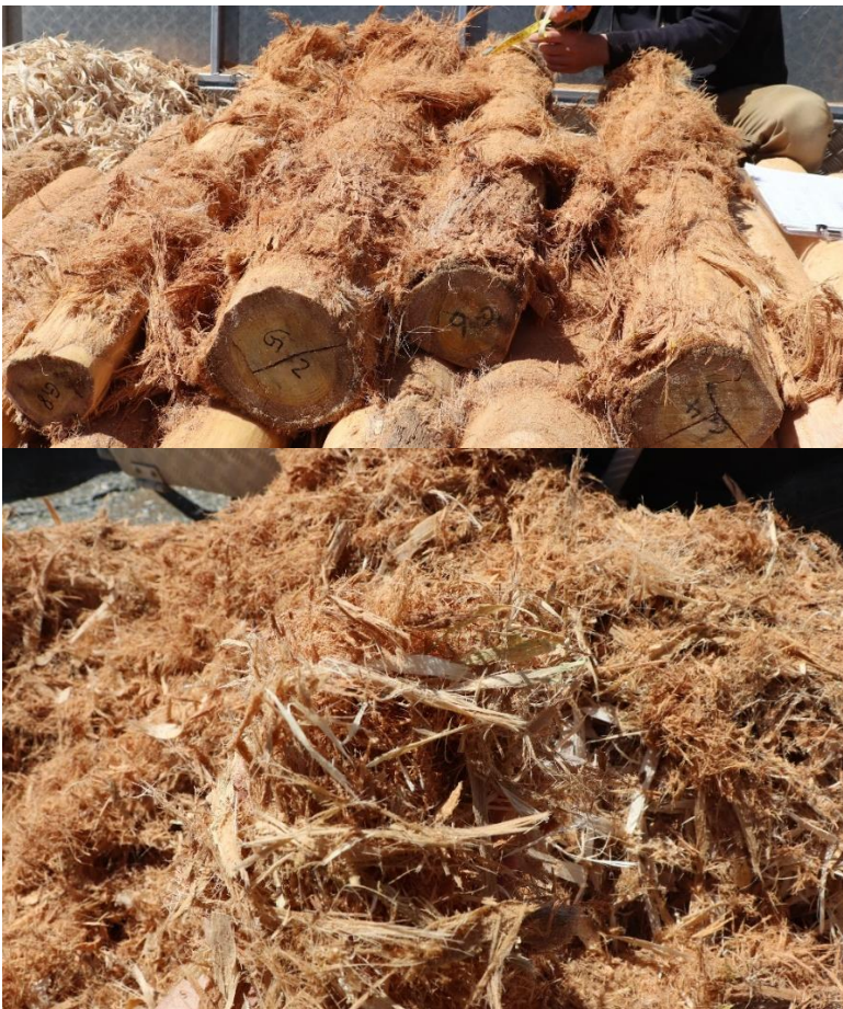
Figure 9: E. globoidea logs with bark after the first pass through the Schälprofi 500 (Posch) (top) and a representative sample of the bark shavings (bottom).
