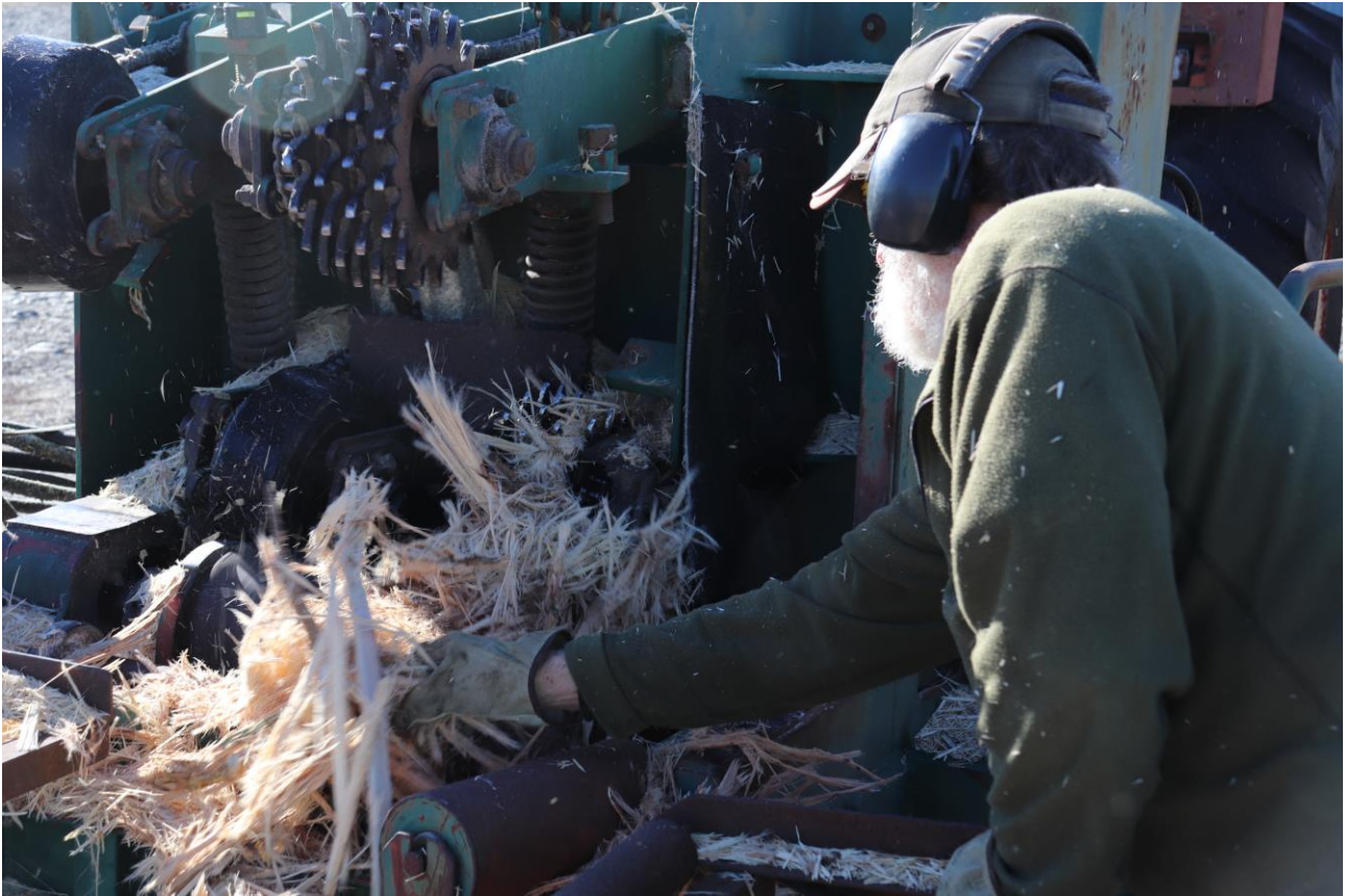
Figure 15: E. bosistoana bark strips jamming the log infeed of the Morbark post peeler.
