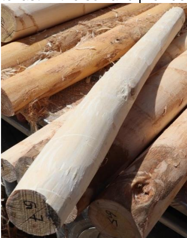
Figure 11: After passing an E. globoidea log (G7) five times through the Schälprofi 500 (Posch) most sapwood was removed.
