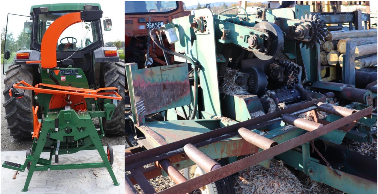
Figure 4: Posch Schälfprofli 500 (left) and Morbark (right) post peeler used for durable eucalypts trials.
