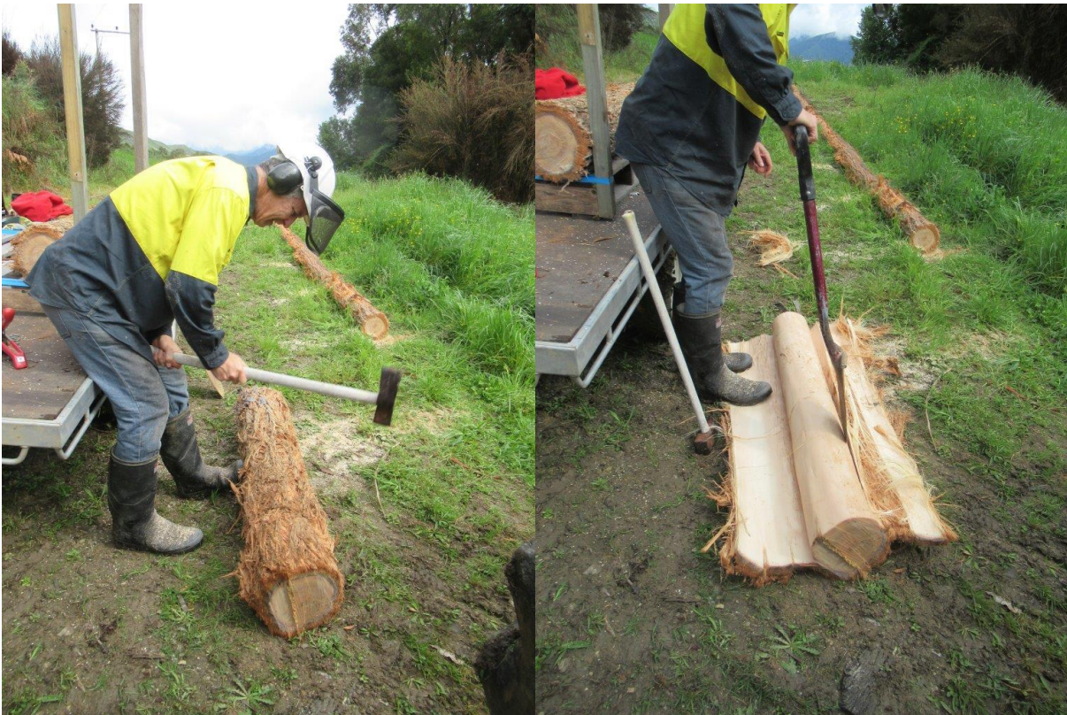
Figure 1: Debarking E. globoidea log shortly after felling by first bruising with a sledge hammer and then stripping the bark with a spade.
