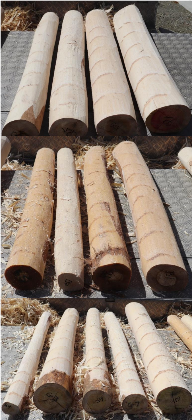
Figure 5: Debarked logs after one pass through the Schälprofi 500 (Posch). E. quadrangulata , E. bosistoana and E. globoidea (from top to bottom).
