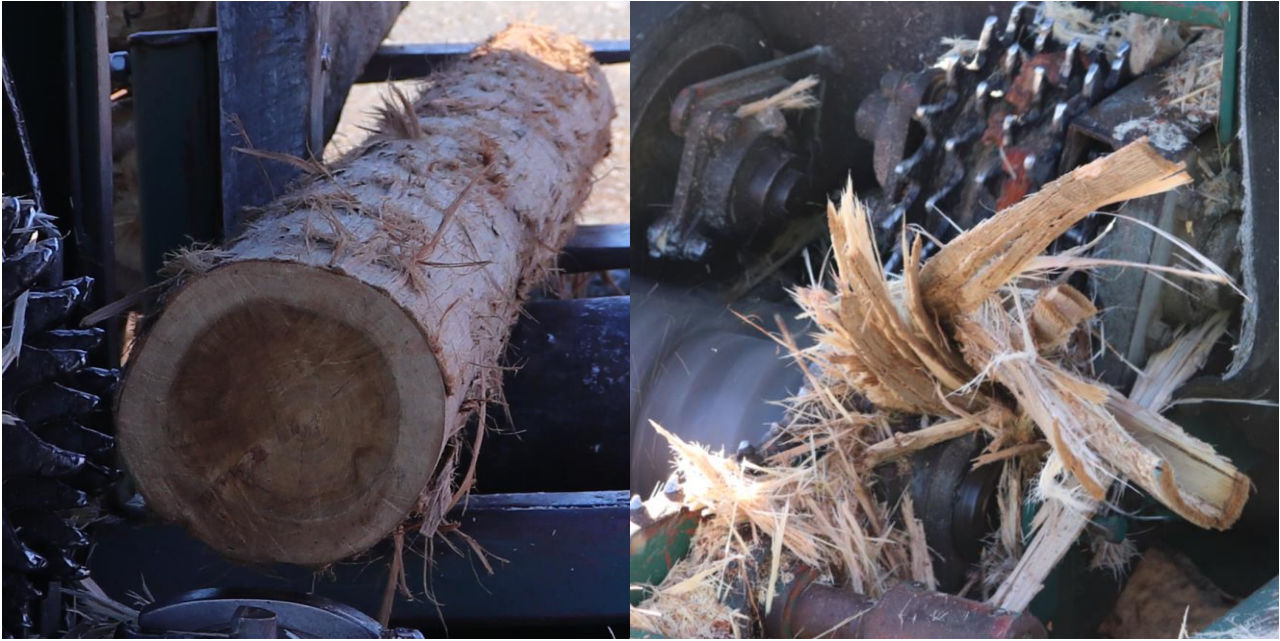
Figure 19: Left - Not cleanly debarked E. bosistoana (3B1) log with a thin layer of inner bark attached (left). Right - inner bark caught up in the log infeed of the Morbark post peeler.
