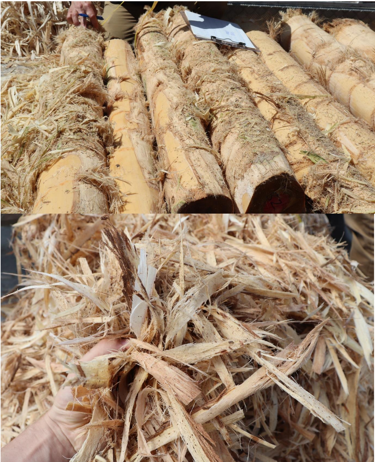
Figure 7: E. quadrangulata and E. bosistoana logs with bark after one pass through the Schälprofi 500 (Posch) (top) and a representative sample of the bark shavings (bottom).
