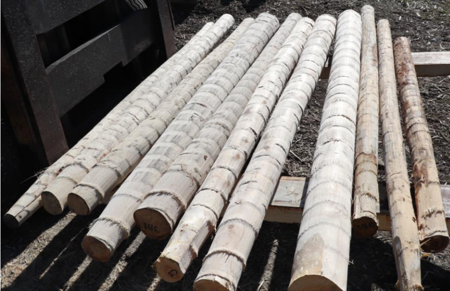
Figure 17: Posts produced with the Morbark post peeler. Note the tapered log ends.
