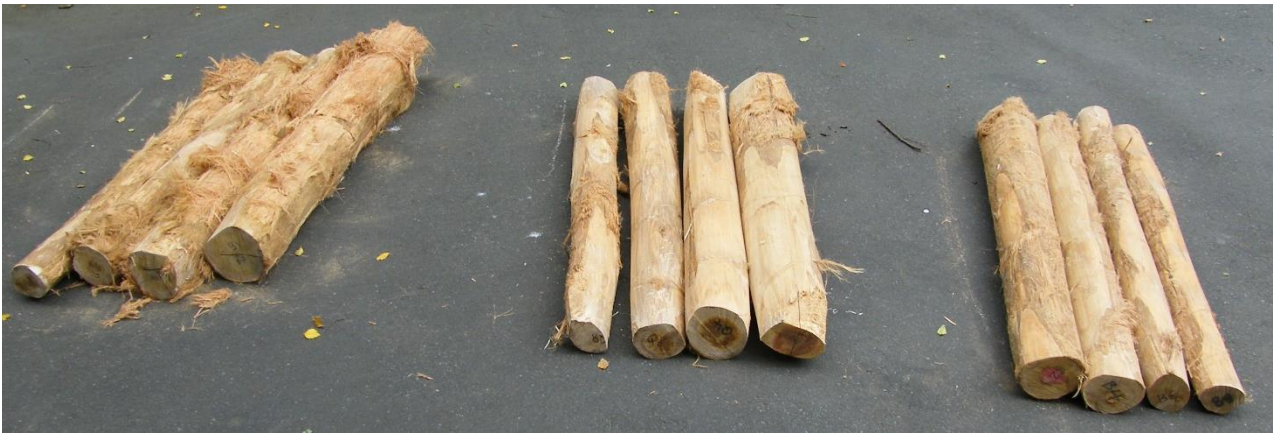
Figure 8: E. globoidea (left), E. quadrangulata (middle) and E. bosistoana (right) logs with bark after two passes through the Schälprofi 500 (Posch).
