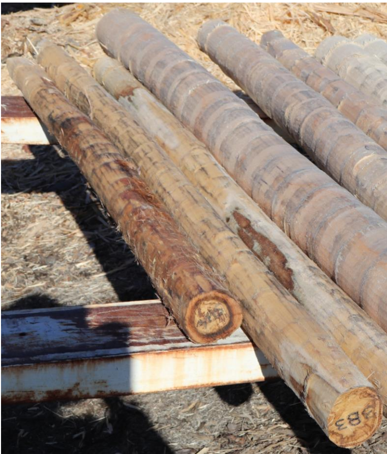
Figure 16: Undebarked E. bosistoana logs: after 1 pass through the Morbark post peeler (3B5 – short post on the left). Note sapwood has not been peeled. After 2 passes through the Morbark post peeler (3B3 and post to the right (2B2)) sapwood was removed.
