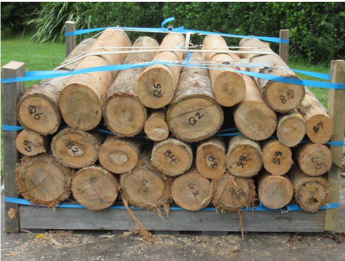
Figure 2: 1.2 m long logs from one tree of each, E. bosistoana , E. quadrangulata and E. globoidea , were used for post peeling with the Schälprofi 500 (Posch). Every second log along the stem was manually debarked in the forest (see Figure 1).
