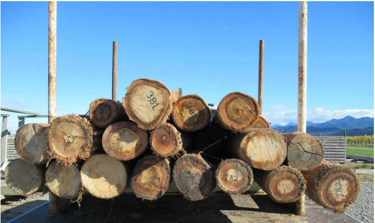
Figure 3: 2.4 m long debarked and undebarked logs used for post peeling with the Morbark equipment.
