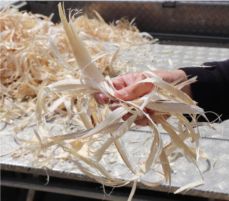
Figure 6: Sapwood shavings produced by the Schälprofi 500 (Posch) from debarked durable eucalypt logs.
