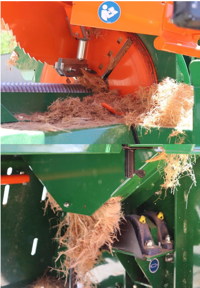
Figure 10: Fibrous E. globoidea bark accumulating in the knife disk (left) and under the operating table (right) after the 1 st pass of the not debarked E. globoidea logs.
