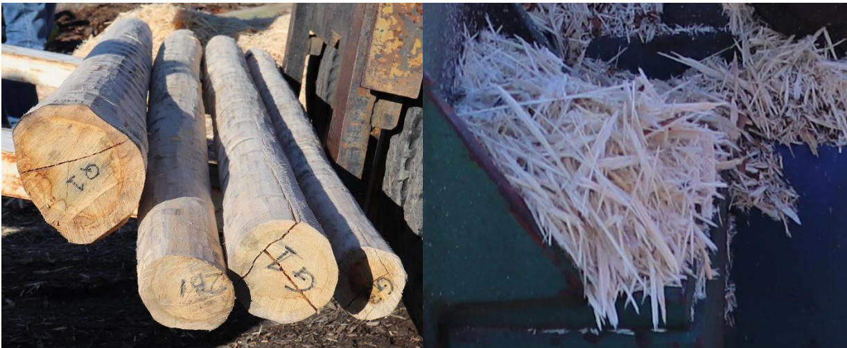
Figure 13: Left: Debarked logs after one pass through the Morbark post peeler. E. quadrangulata (Q1), E. bosistoana (2B1) and E. globoidea (G1 and G3). Right: Sapwood shavings produced from debarked durable eucalypt logs.
