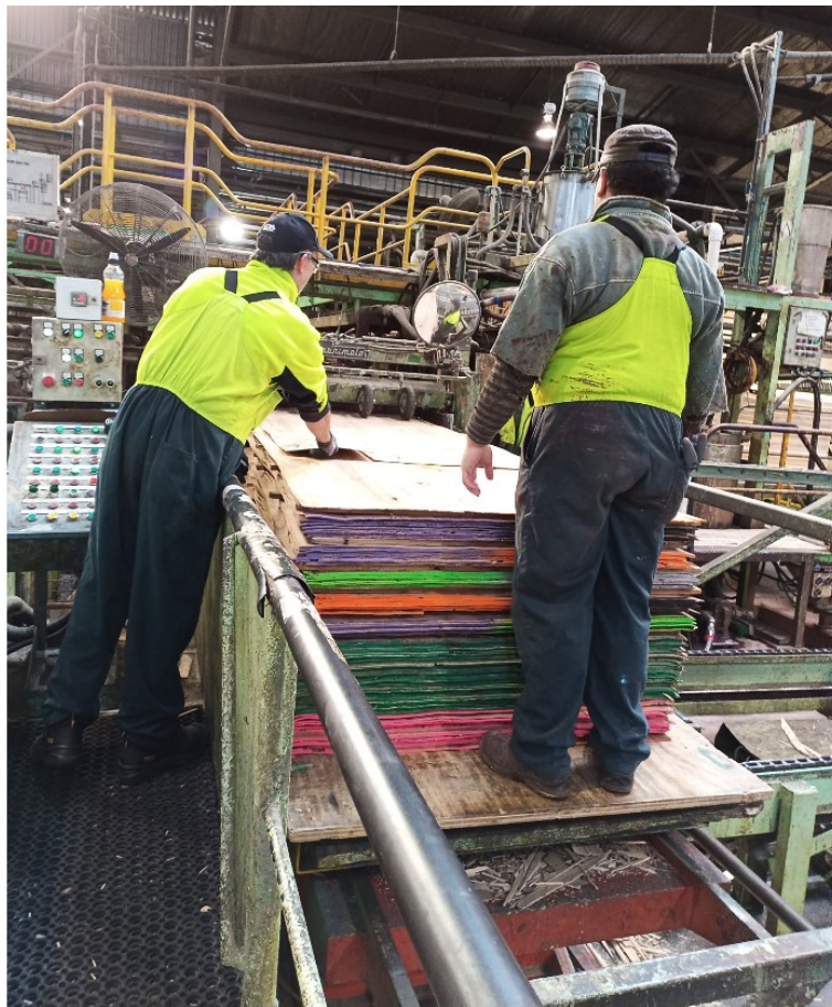
Figure 1. Colour coded veneer sheets are fed into the glue spreader
