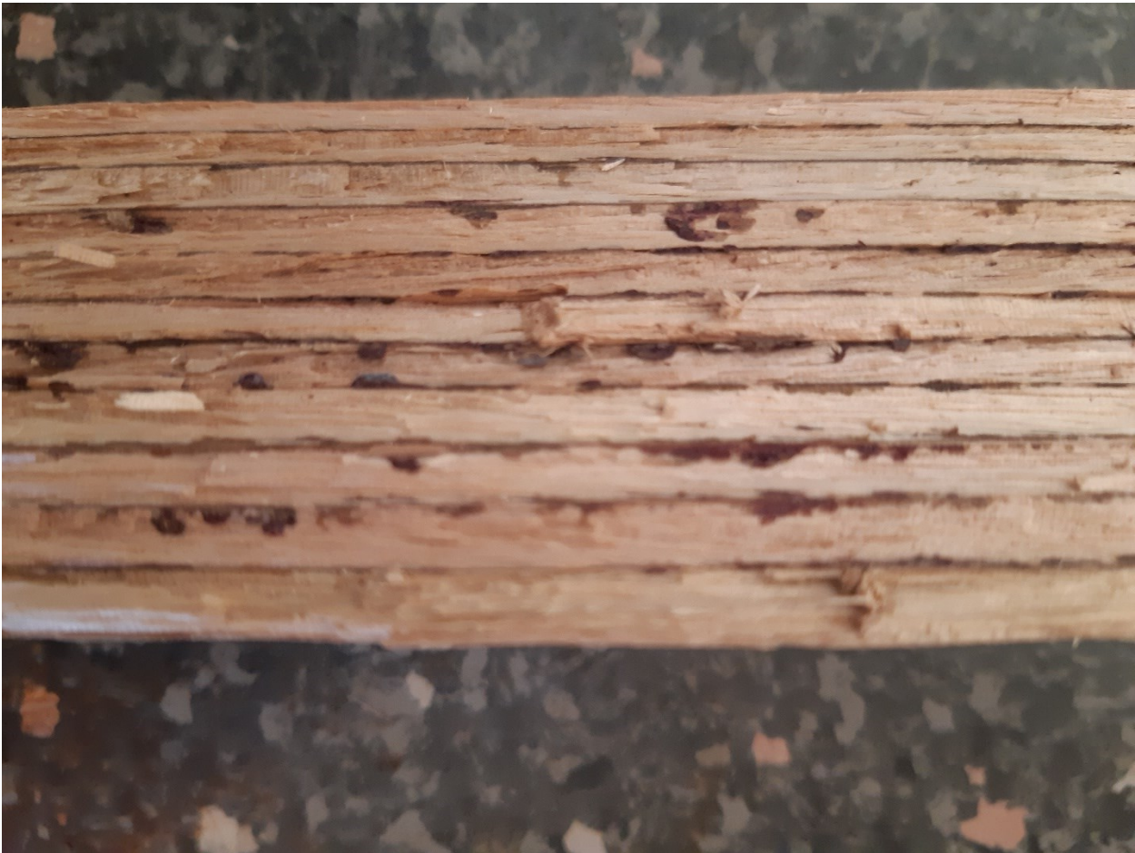
Figure 11. Evidence of splits within the veneers
