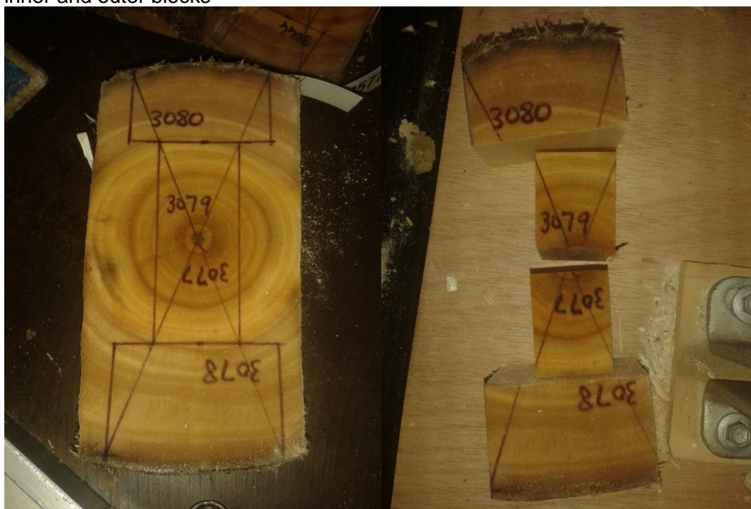
Figure 1. Picture of blocks cut in previous study showing location within disk and positioning of inner and outer blocks
