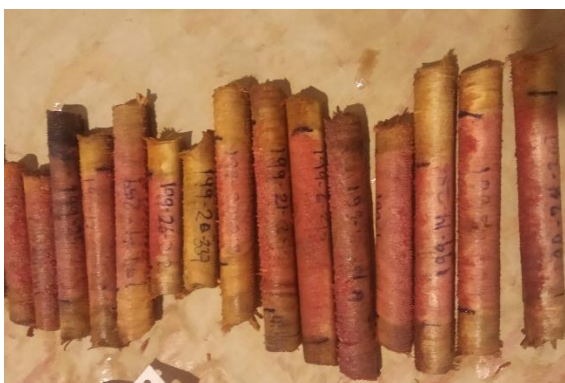
Figure 3: E. globoidea cores with heartwood dyed pink after application of methyl orange.
