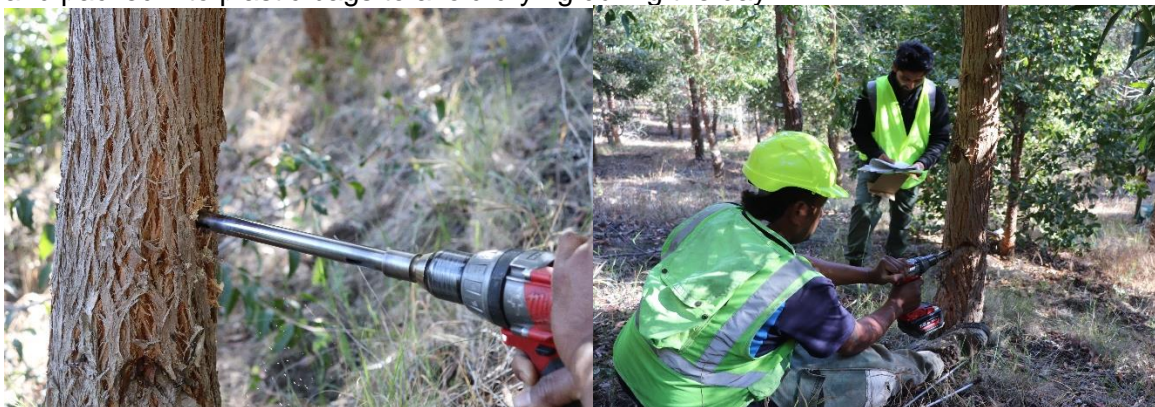
Figure 2: Coring an E. globoidea tree at Avery using a battery-powered 14 mm diameter corer
