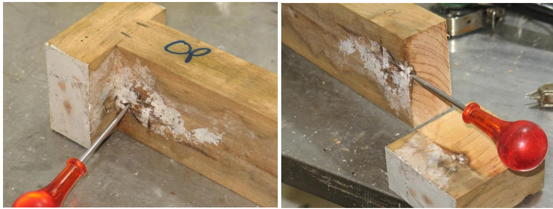
Figure 9: Decay on the surface and in the joint of an untreated Cupressus macrocarpa sample from an old tree, after one year's exposure (sample 84).
