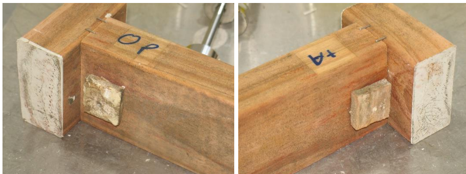
Figure 14: No decay and moderate mould on a boron treated radiata pine sample after one year's exposure (sample 80).
