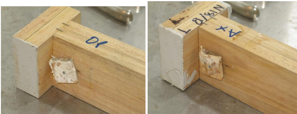
Figure 7: No mould, mycelium or decay on the surface of boron treated Eucalyptus nitens sample after one year's exposure (sample 47).
