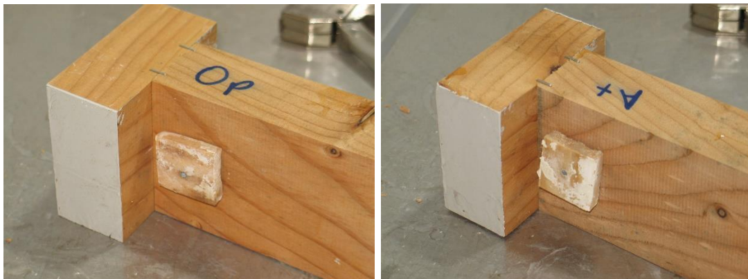
Figure 11: No mycelium or mould growth, or decay, on an untreated Larch sample after one year's exposure (sample 115).
