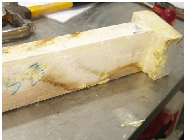
Figure 5: Extensive mycelium over half of the surface of an untreated Eucalyptus nitens sample after one year's exposure (sample 53).
