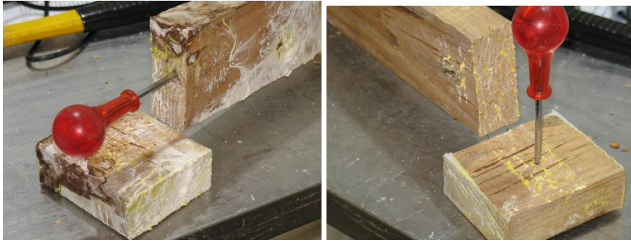
Figure 12: Well established decay in the joints of an untreated Douglas fir sample after one year's exposure (sample 125).
