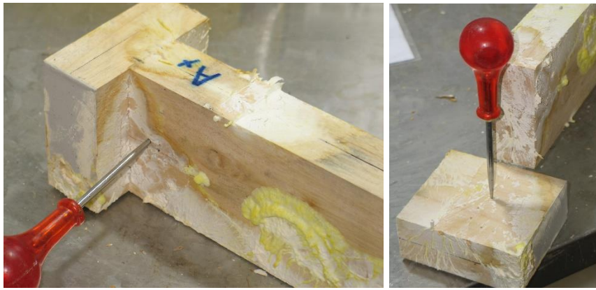
Figure 6: Lightly established decay on the surface and in the joint of an untreated Eucalyptus nitens sample after one year's exposure (sample 57).
