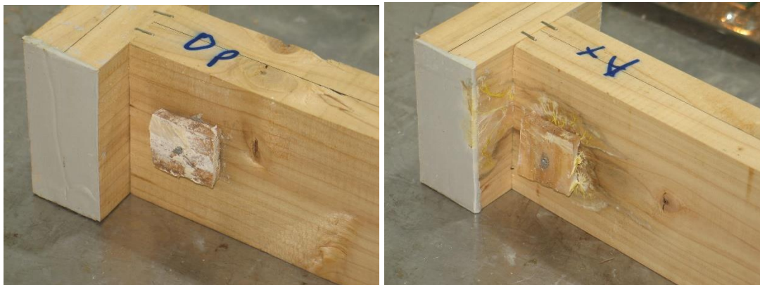
Figure 10: No mycelium growth at the Op feeder block and moderate mycelium growth at the Ax feeder block of an untreated Cupressus x ovensii sample after one year's exposure (sample 108).
