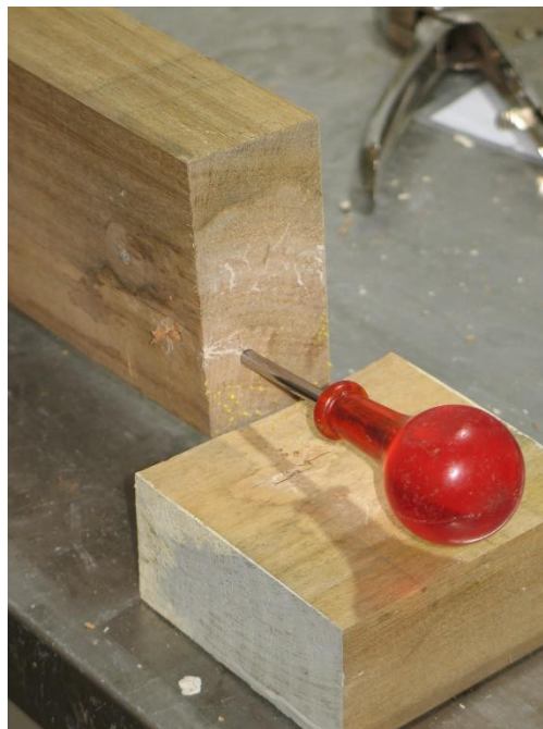
Figure 2: Severe decay in the joint of untreated Eucalyptus fastigata after one year's exposure (sample 13).
