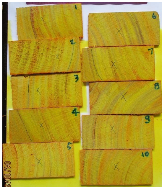
Figure 16: Penetration \sap spot test images of Eucalyptus fastigata in cross section
