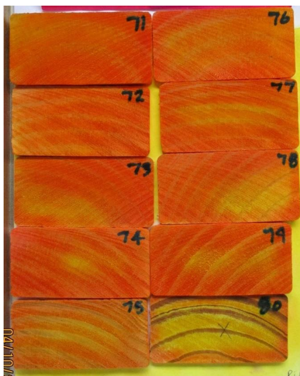
Figure 22: Penetration \sap spot test images of radiata pine in cross-section
