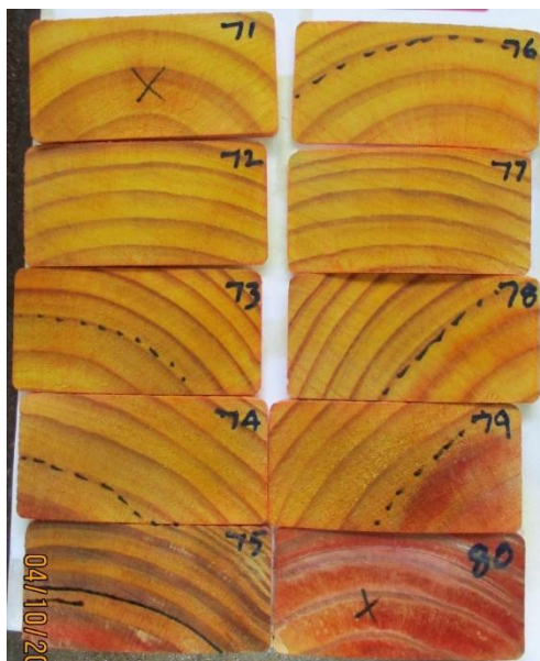
Figure 21: Heart\sap spot test images of radiata pine in cross section
