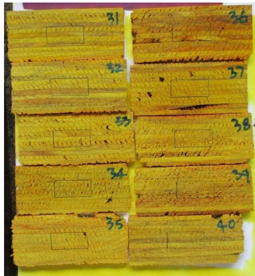
Figure 18: Penetration \sap spot test images of Eucalyptus fastigata LVL in cross section
