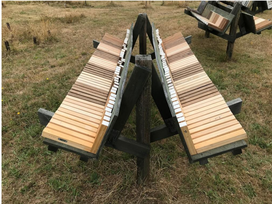
Figure 1: General view of L-joint trial at the time of installation (February 2022).
