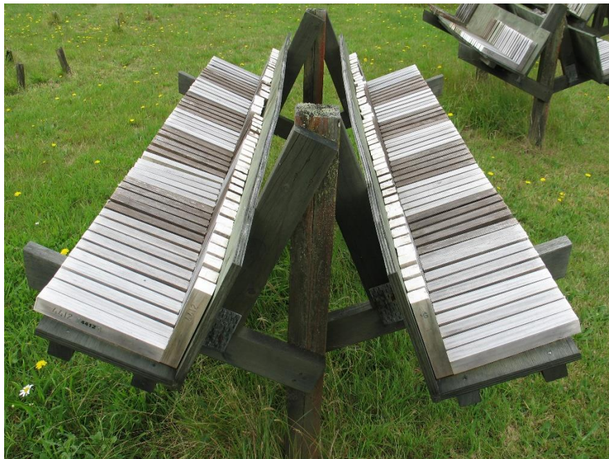
Figure 2: General view of L-joint trial after one year's exposure (February 2023).
