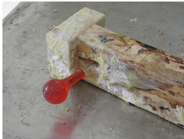
Figure 11: Decay on the surface of an untreated radiata pine sample after eighteen months exposure (sample U2).
