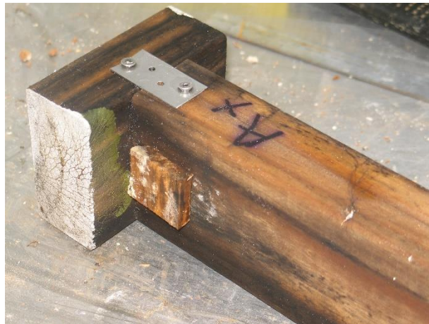
Figure 8: Suspected soft rot on a boron treated radiata pine sample after twenty-four months exposure (sample 604).
