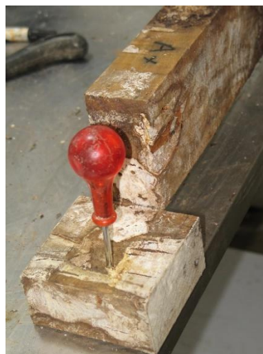
Figure 3: Decay in the joint of a heartwood Cupressus lusitanica sample after twenty-four months exposure (sample 231).
