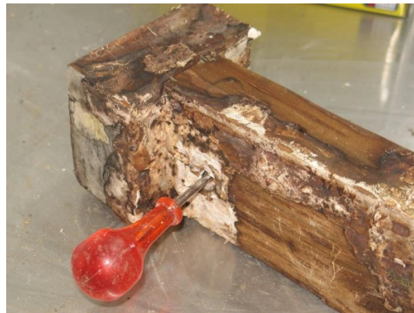
Figure 2: Decay on the surface of a mixed heartwood/sapwood Cupressus lusitanica sample after twenty-four months exposure (sample 207).
