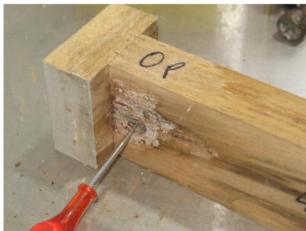
Figure 6: Decay on the surface of a heartwood Eucalyptus regnans sample after twenty-four months exposure (sample 401).
