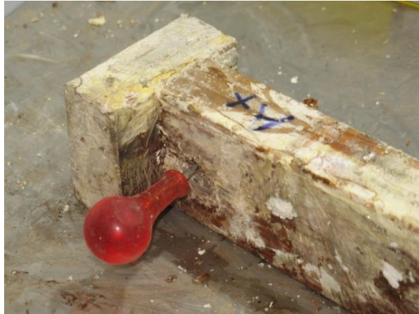
Figure 4: Severe decay on the surface of a Douglas fir heartwood sample after twenty-four months exposure (sample 501).
