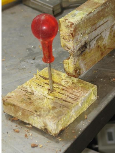
Figure 10: Decay in the joint of a heartwood Eucalyptus nitens sample after eighteen months exposure (sample 810).
