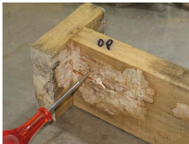
Figure 9: Decay on the surface of a heartwood Eucalyptus nitens sample after eighteen months exposure (sample 801).
