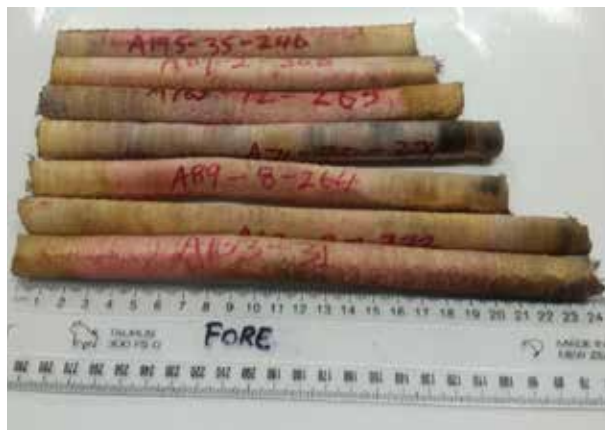
↑ Figure 22: Examples of cores from which heartwood thickness can be measured.
