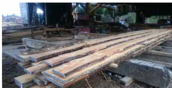
→ Figure 16: Boards sawn from young unpruned cypress, ready to be resawn, air-dried and then graded.
