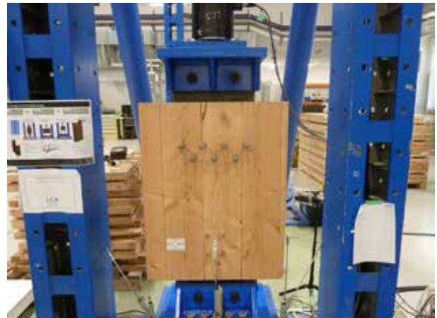
↑ Figure 3: Testing Douglas-fir CLT connections.
