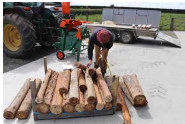
↑ Figure 29: Associate Professor Clemens Altaner assesses durable eucalypt posts peeled by a tractor-mounted machine.
