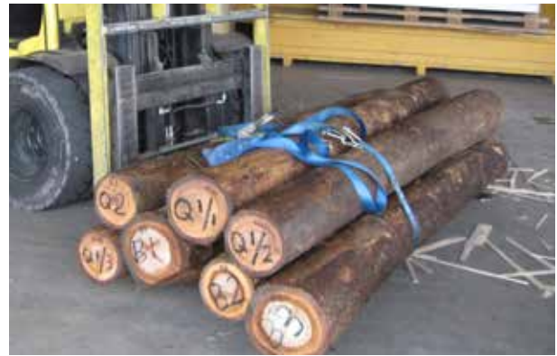
↑ Figure 27: Durable eucalypt logs being delivered to Nelson Pine Industries for peeling to make veneer.
