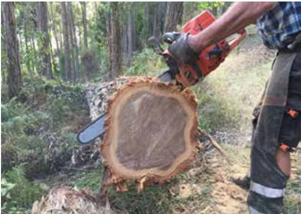
↑ Figure 24: Heartwood is clearly visible in the disc being cut from the tree stem.
