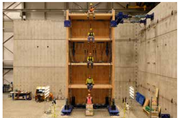
↑ Figure 4: The Douglas-fir CLT structure being tested for seismic resilience in the University of Canterbury engineering lab.
