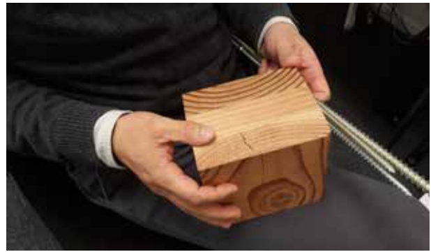
↑ Figure 2: CLT and the screws used to connect the CLT panels.
