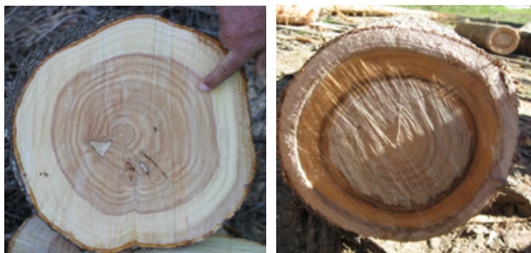
Cross sections of (left) Cupressus macrocarpa and (right) Eucalyptus bosistoana showing the darker, durable heartwood in the centre, and the lighter sapwood band around the outside. C. macrocarpa is moderately durable; E. bosistoana is very durable. Species with a narrow sapwood band yield a greater proportion of heartwood when milled, so this is a desirable trait.
